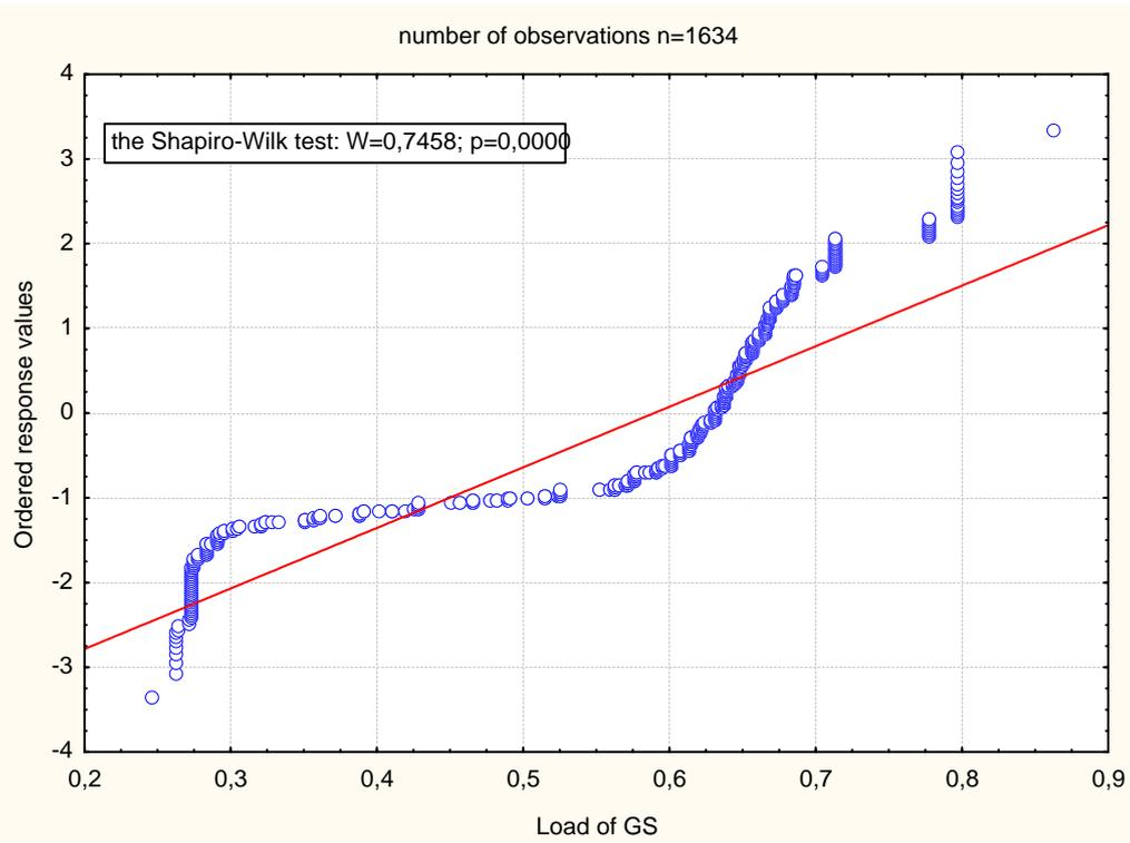
Fig. 3. Normal probability plot and the results of the Shapiro-Wilk test for the generating sets' peak loads of 7500 TEU container ship (IA)
