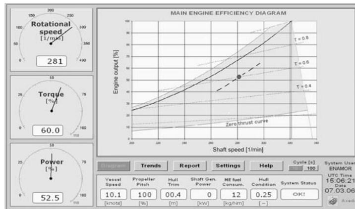
Fig. 2. The main engine efficiency diagram in power plant monitoring system on the training ship m/s “Horyzont II”. Marked point of actual working state of main engine
