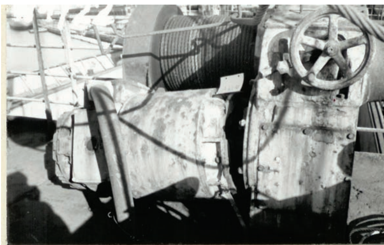
Fig. 3. Electric driving motor torn off the hoisting winch body
