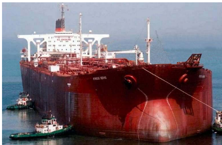
Fig. 1. ULCC class tanker Knock Nevis: length 458,45 m, 564763 DWT
