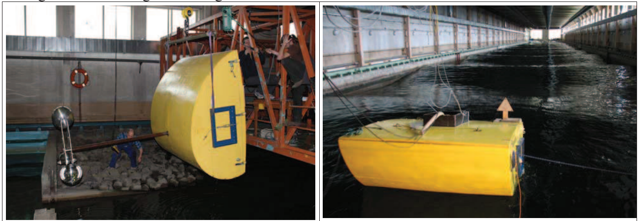
Fig. 5. Photographs of the power buoy model - on the left during preparation for launching, on the right during tests in the towing tank
