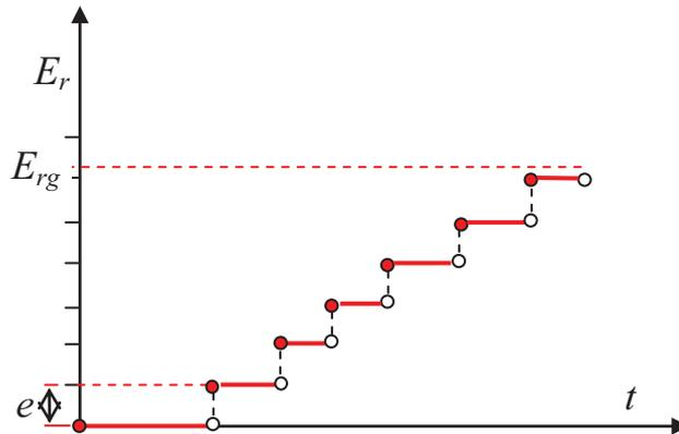
Fig. 1. Interpretation of the process of accumulating dissipated energy  $E_r$  for a machine (power system):  $e$  – portion of energy (quantum), by which the energy  $E_r$  decreases,  $E_{rg}$  – boundary dissipation energy
