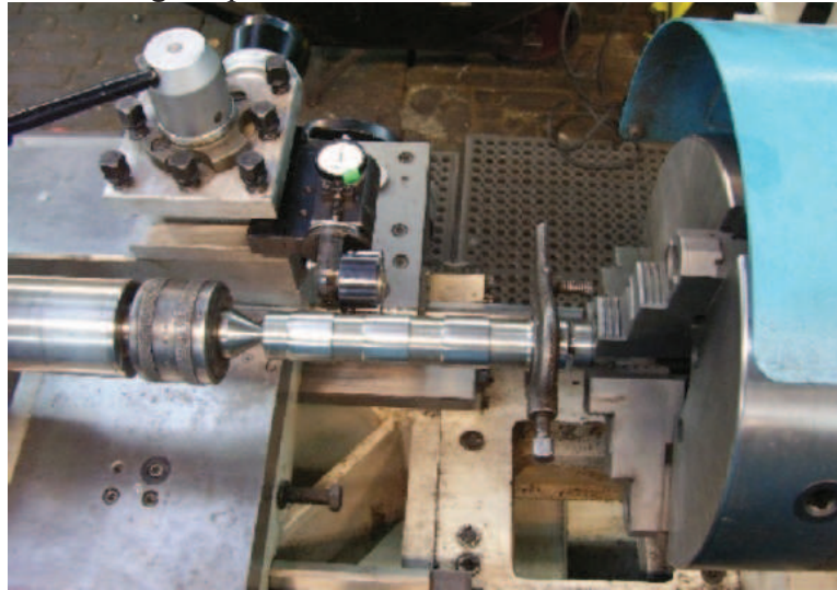
Fig. 3. General view of OUPN tooling system (machine, grip, object, tool): burnishing
