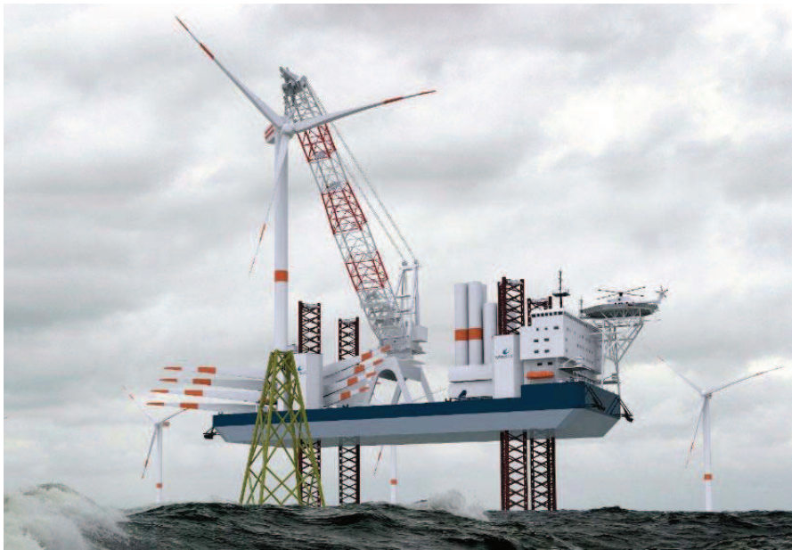
Fig. 8. Jack-up barge for installation of offshore wind farm
