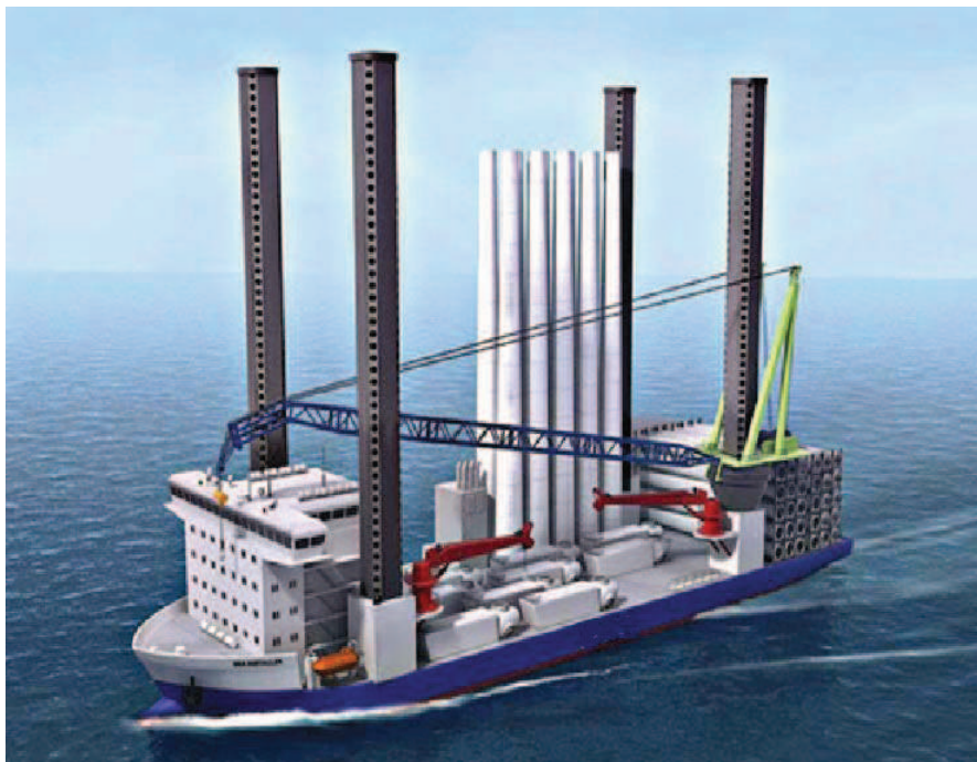
Fig. 9. Ship shaped vessel for transportation and installation of offshore wind farm
