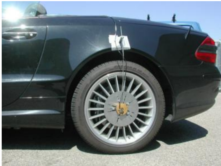
Fig.2. Manner of fixing a measurement disc with the sensor
