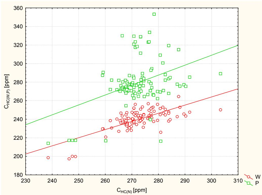
Figure 4. The concentration of hydrocarbons HC for the transient at  $n = 1100 \text{ r / min}$  and load change from  $T_{iq} = 30 \text{ N}$  to  $T_{iq} = 50 \text{ N}$ : P - late, W - accelerated injection timing, CHC (N, S, P) - HC concentration for (N) nominal, (W) accelerated, (P) delayed injection timing
