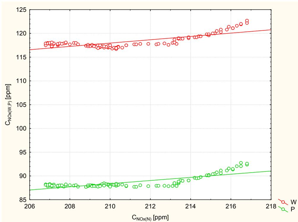
Figure 5. The concentration of NOx for the transient at  $n = 1100 \text{ r / min}$  and load change from  $T_{iq} = 30 \text{ N}$  to  $T_{iq} = 50 \text{ N}$ : P - late, in - accelerated injection timing, CNOx (N, S, P) - NOx concentration (N) nominal, (W) accelerated, (P) delayed injection timing
