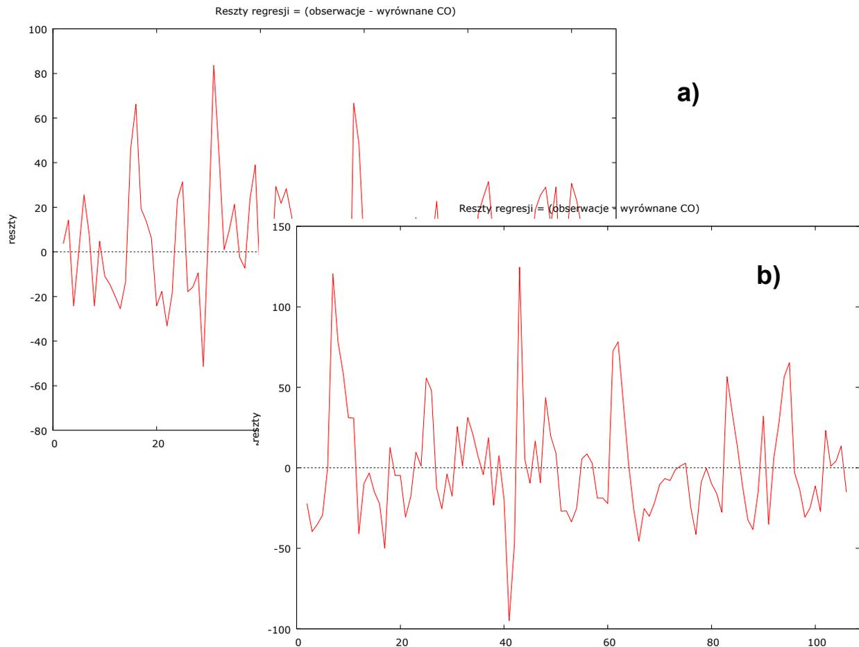
Figure 3. Graph of the CO regression residuals for the transient at  $n = 1100 \text{ r/min}$  and load change from  $T_{tq} = 50 \text{ N}$  to  $T_{tq} = 70 \text{ N}$  a) delayed (P) injection timing, b) accelerated (W) injection timing.
