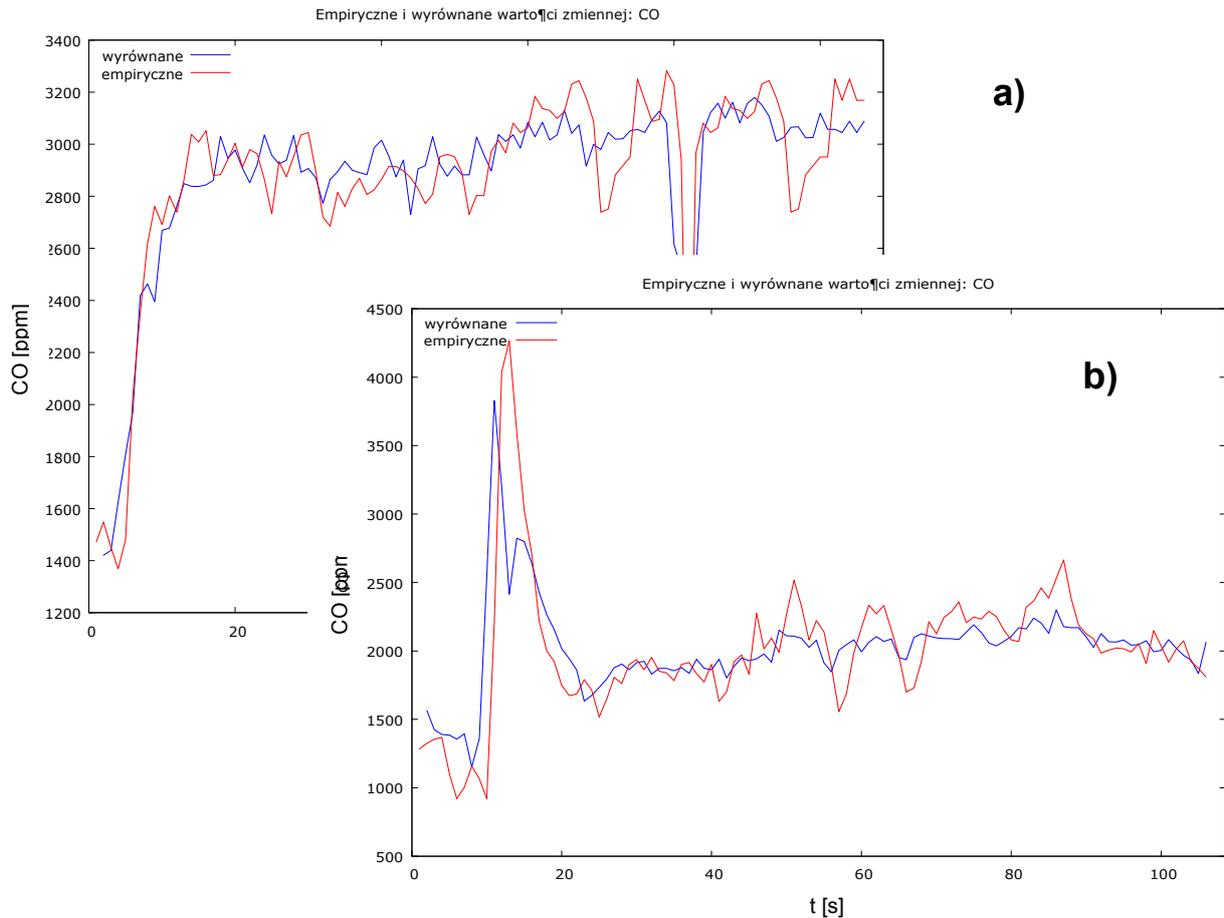
Figure 2. Graphical matching of the CO model to the empirical data for the transient at  $n = 1100$  r / min and load change with  $Ttq = 50$  to  $N = 70$  N Ttq a) delayed (P) injection timing angle, b) accelerated (W) injection timing angle
