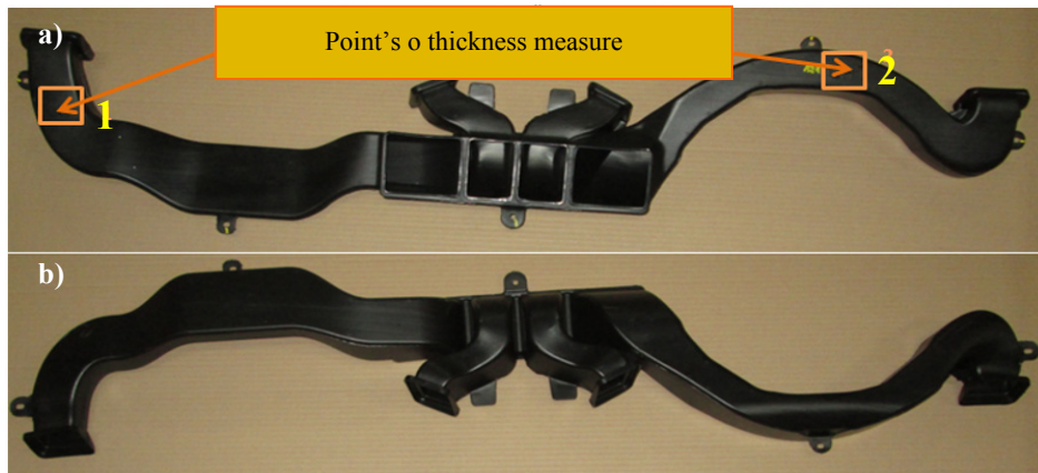
“Fig. 3. Finish blowing products: a)critical measure points – side view, b) product top view”
