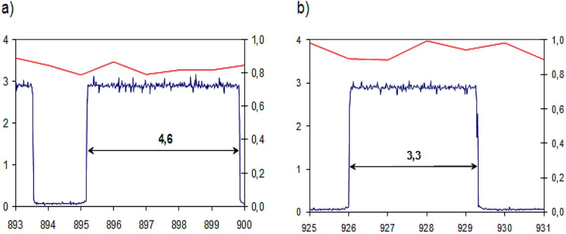
Pic.6a)Duration of energy impulse at low vibrations level b)Duration of energy impulse at high vibrations level
