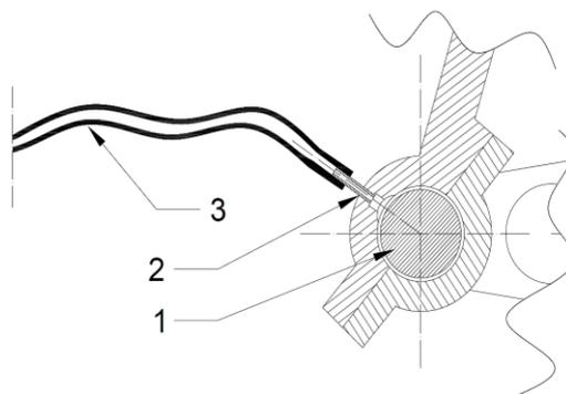
*Pic.3. Detailed lubrication system of crank bearing.*
