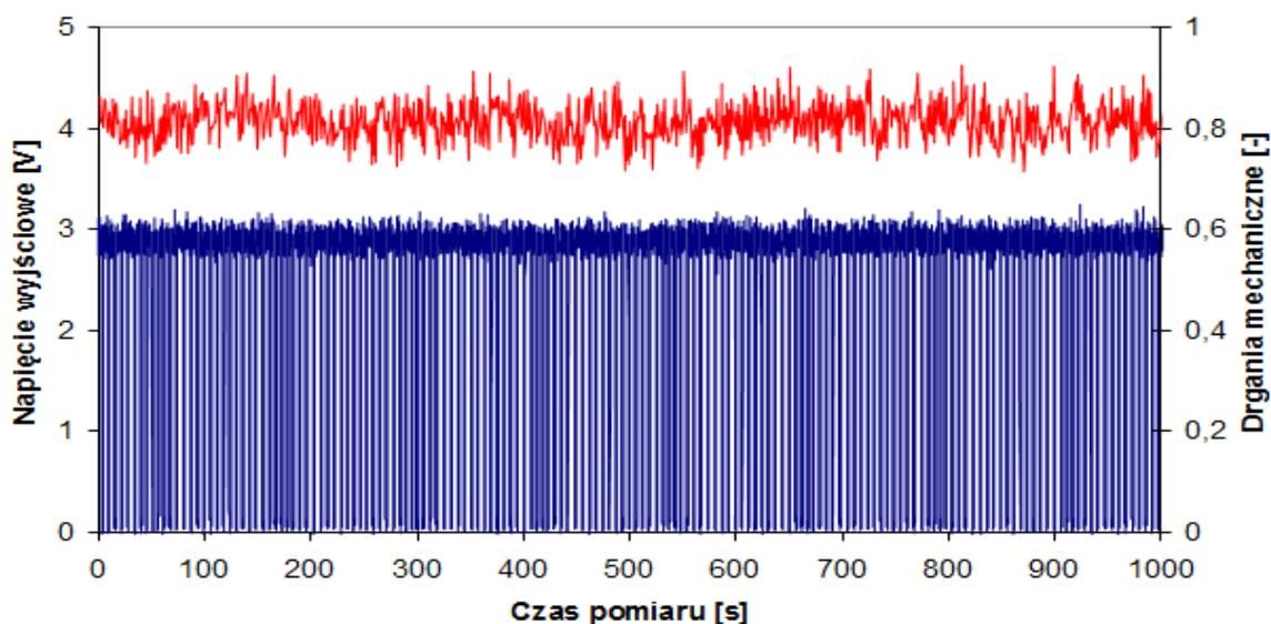
*Pic.4 Change of course of voltage of measure impulses and vibration's level characteristic for operation of side bearing for stage A*
