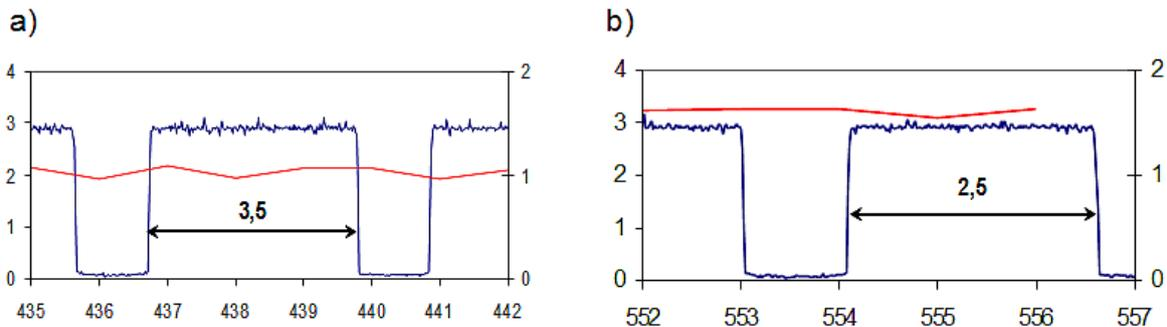
Pic.10 a)Duration of energy impulse at low vibrations level b)Duration of energy impulse at high vibrations level
