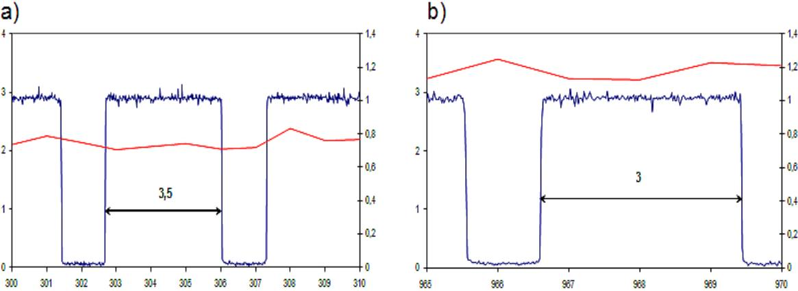
Pic.8a)Duration of energy impulse at low vibrations level b)Duration of energy impulse at high vibrations level
