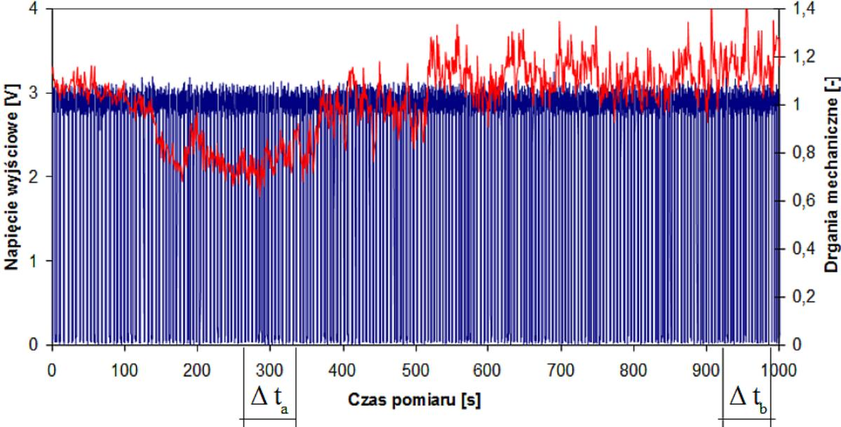
Pic.7. Change of course of voltage of measure impulses and vibration's level characteristic for operation of side bearing for stage C
