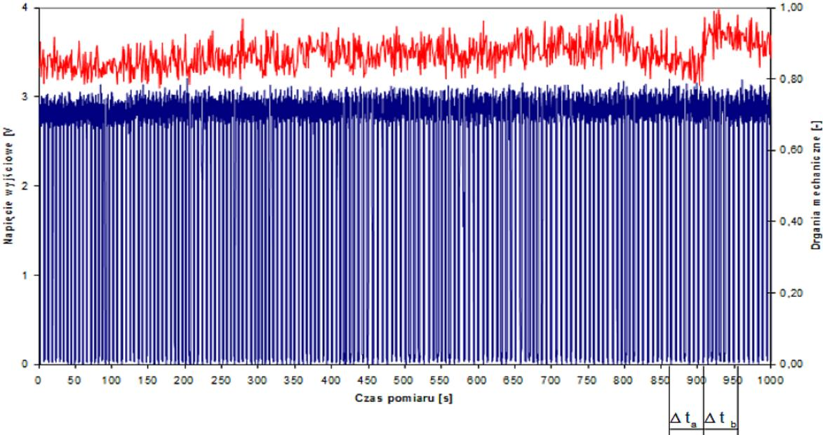
Pic.5 Change of course of voltage of measure impulses and vibration's level characteristic for operation of side bearing for stage B
