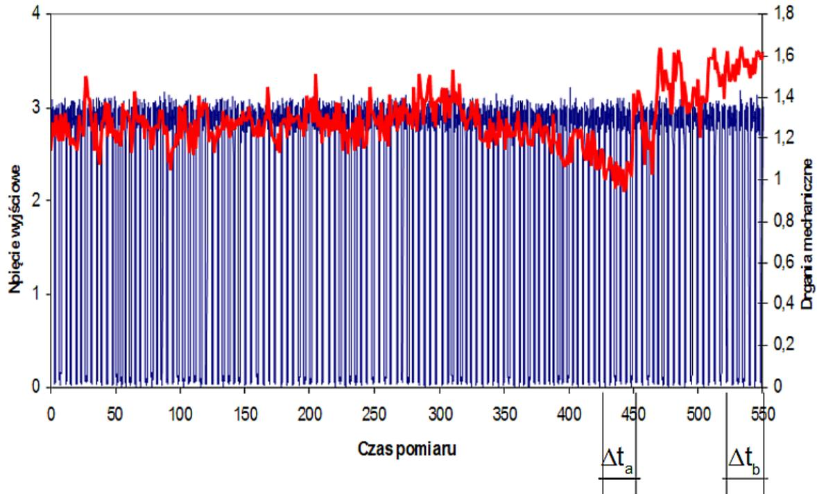
Pic.9. Change of course of voltage of measure impulses and vibration's level characteristic for operation of side bearing for stage D
