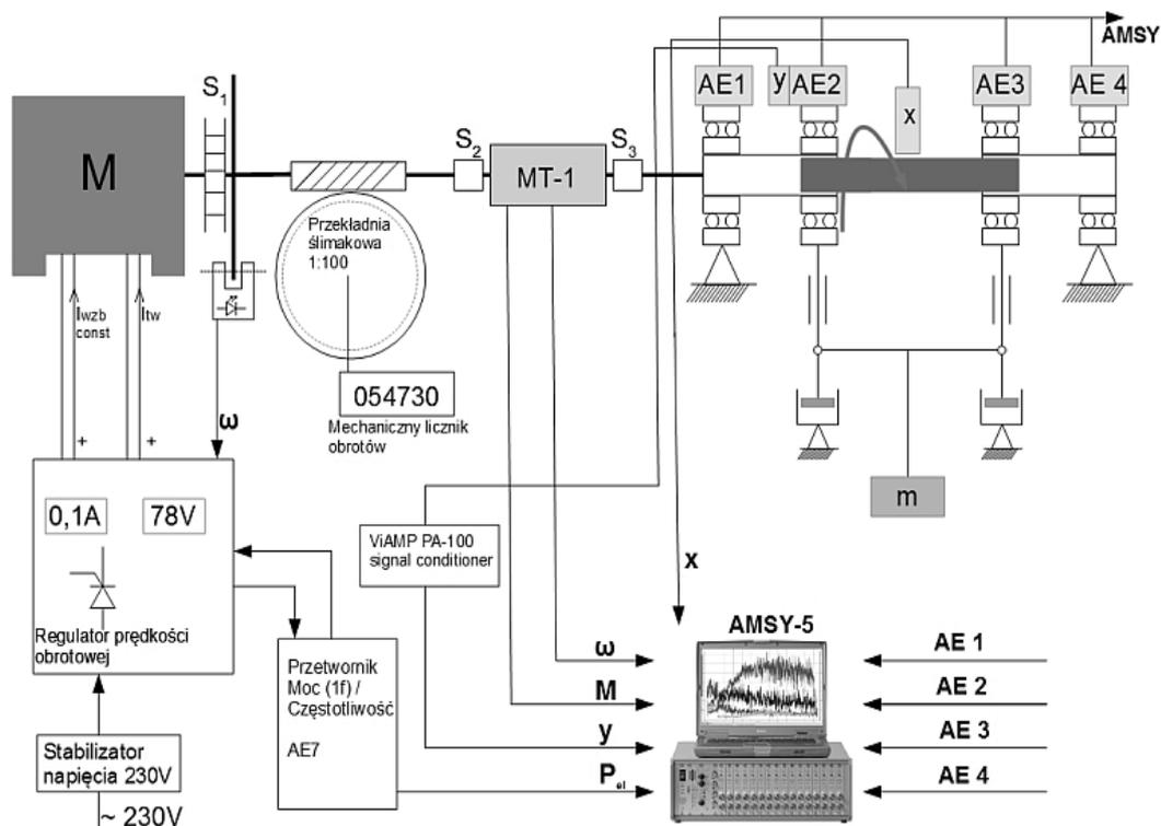
*Pic. 2. Physical model of rotating transmission system: M – electric motor 0,25kW; MT-1 – momentum meter; AE1-AE4 – active sensors of acoustic emission; y – accelerometer ; x – bending sensor; S<sub>1</sub>-S<sub>3</sub> – flexible coupling*
