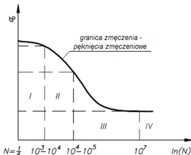
Pic. 1. Complete<sup>3</sup> Wöhler's graph with identified range of a fatigue durability [Kocańda & Szala, 1985]: I - quasi-static; II - low-cycle; III - high-cycle; IV - unlimited fatigue durability
