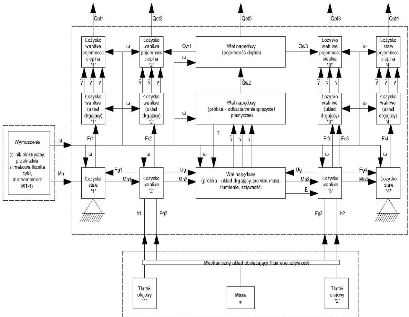
Pic. 5. Physical model of energy-related processes realised in the considered physical model:  $b$  – suppression coefficient,  $Fr$  – radial forces,  $Fg$  – load forces,  $Fo$  – axial forces,  $\omega$  – angular velocity,  $Mn$  – momentum,  $Ug$  – bending of the sample,  $m$  – load mass,  $y$  – acceleration, velocity and dislocation of oscillations;  $Q$  – heat stream emitted to the surroundings
