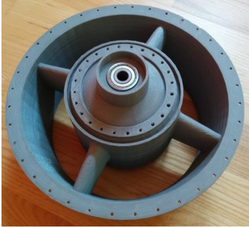
Fig. 12. Mounted ball bearing in engine unit
