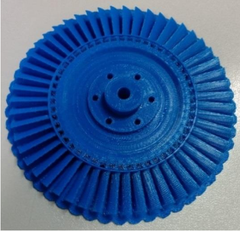
Fig. 7. Power turbine after its extraction from the inside of the Replicator 18
