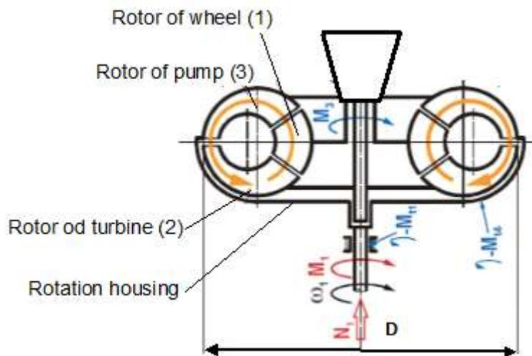
Fig. 1. Scheme of one range torque converter mixer
