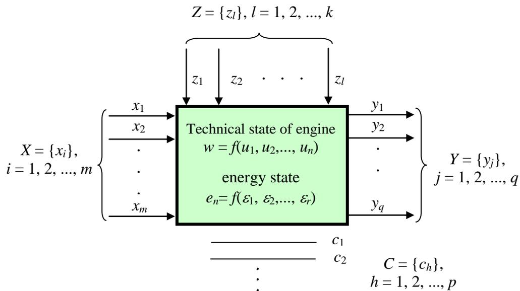
Fig. 1. Operation process for a marine main engine driven by an adjustable-pitch propeller:  $X$  - set of input values,  $w$  - technical state (characterized by parameters of state  $u_i, i = 1, 2, \dots, n$ ),  $e_n$  - energy state (characterized by parameters of state  $\varepsilon_j, j = 1, 2, \dots, r$ ),  $Y$  - set of output values,  $Y$  - set of output variables (diagnostic parameters),  $C$  - set of constant values,  $Z$  - set of interference values (deterministic and random).
