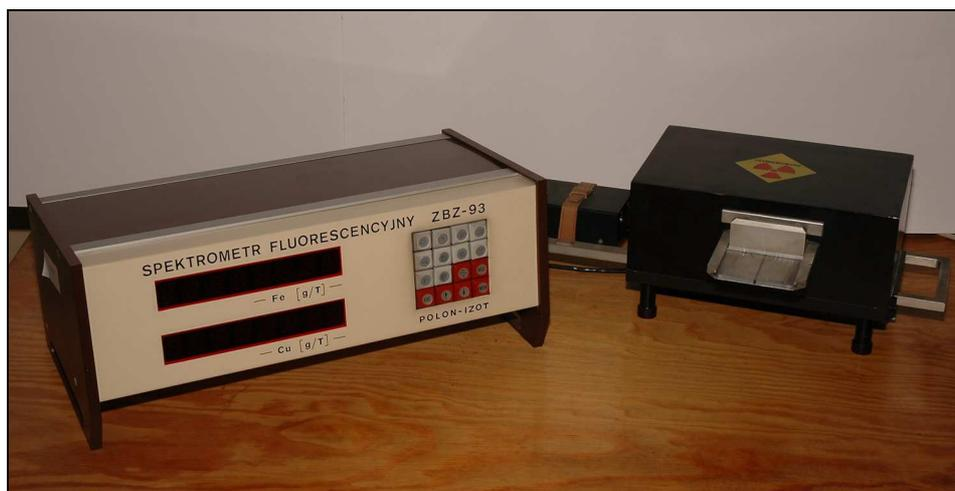
Fig.5. The fluorescence spectrometer ZBZ-93
