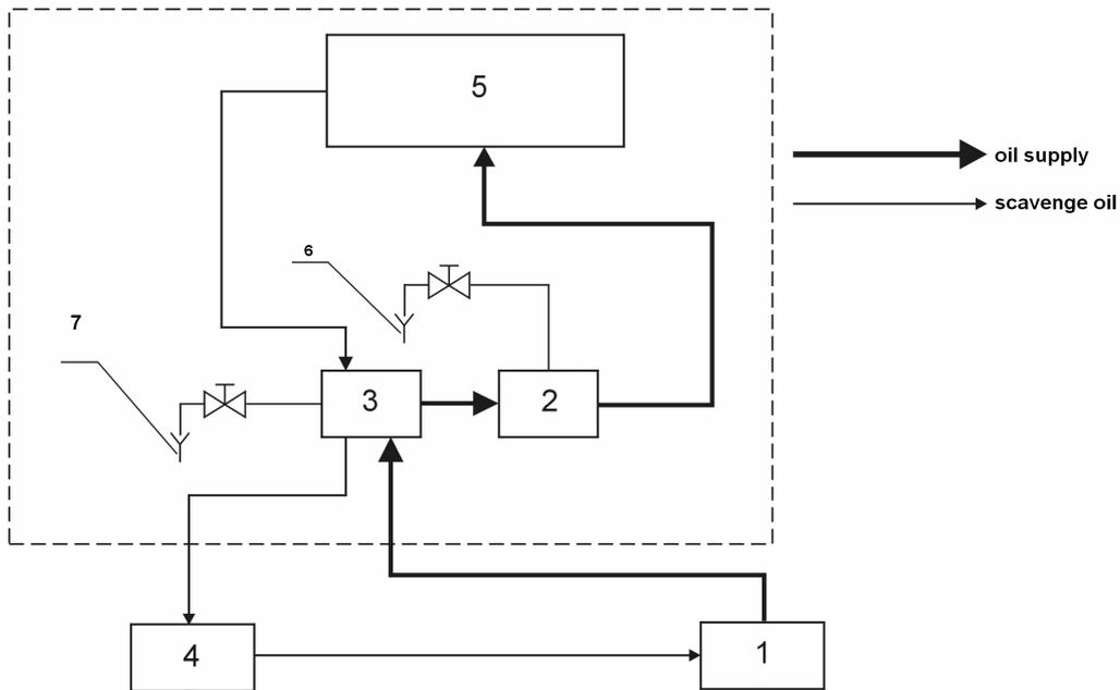
Fig.7. The lube oil system block diagram with the marked places to take oil samples;
