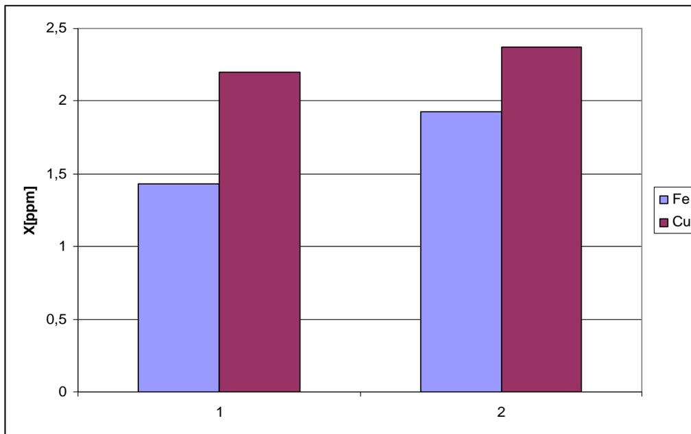
Fig. 8. The graph of Fe and Cu impurities in oil taken from chosen places of oil system:
