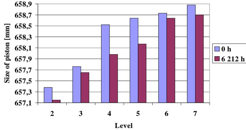
Fig. 7. Changes of pistons dimensions in the direction perpendicular to engine axis for different times of measurements
