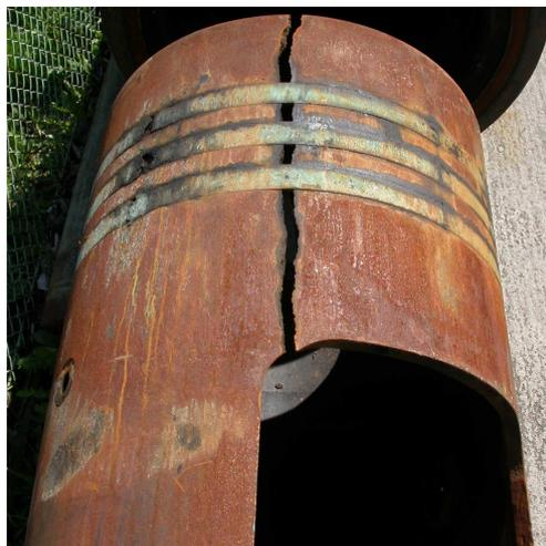
Fig 1. View of a cracked of piston skirt
