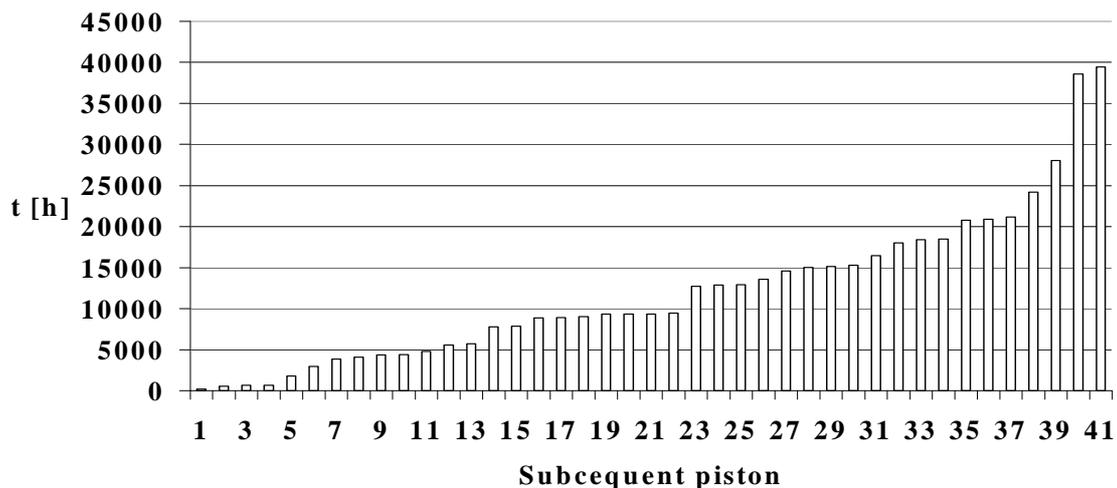
Fig. 3. Well-ordered realizations of time to failure of examined pistons engines, type 6RRLB66
