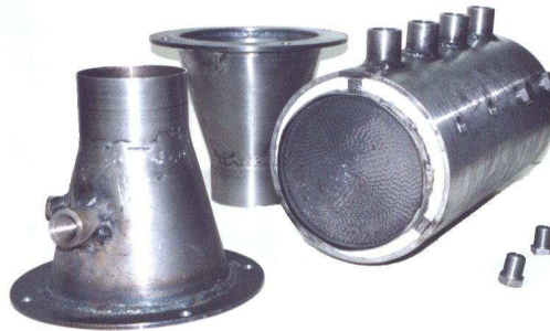
Fig. 6. Metallic enclosure of tested catalytic converter [3]
