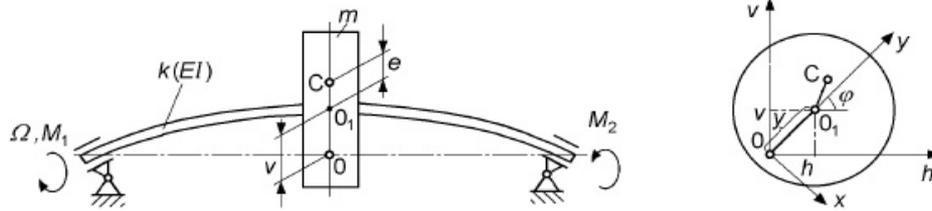
Fig. 1. A simplified shaft-line model for critical speed calculation [4]
