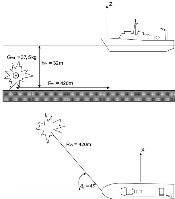
Fig. 3 Schematic diagram of the performed experimental test
