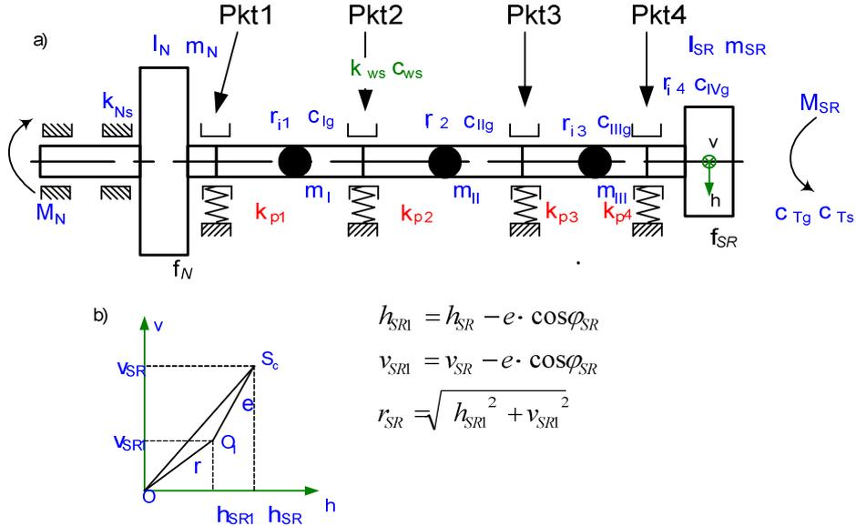
Fig. 9 Scheme of shaft line of minehunter, where:
