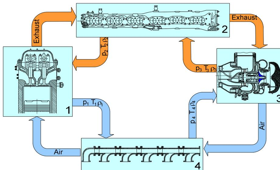
Fig. 1. The relation between particular engine's workspace areas
