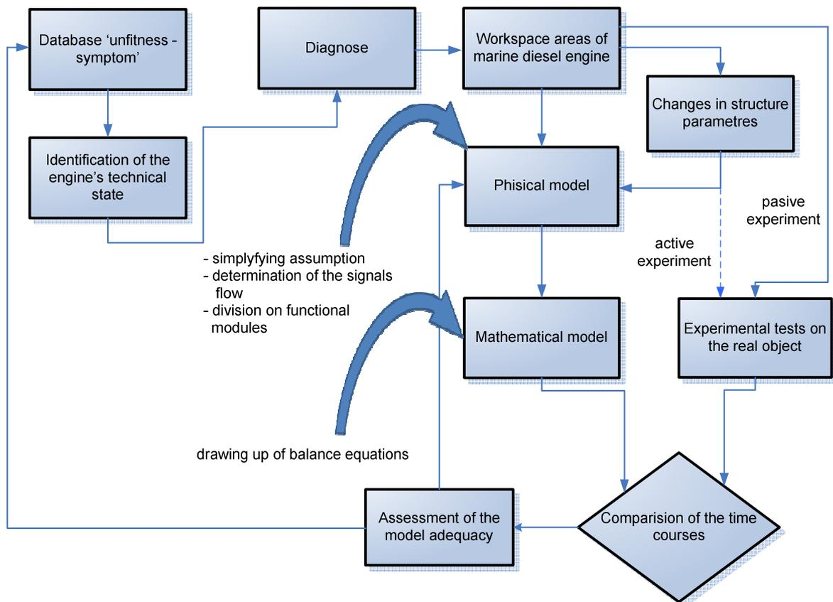
Fig. 5. The research scheme of gasdynamical processes examinations for diagnostic purposes of marine diesel engines
