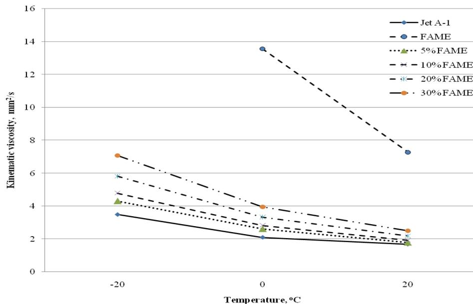
Figure 3. Viscosity change vs. temperature of aviation fuel, FAME and their mixtures
