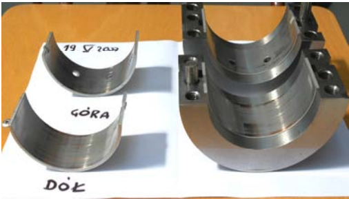
Fig. 14 The view split bearing bushings of the type MB10 and MB35 after investigations visible first traces the waste of the sliding layer [14]
