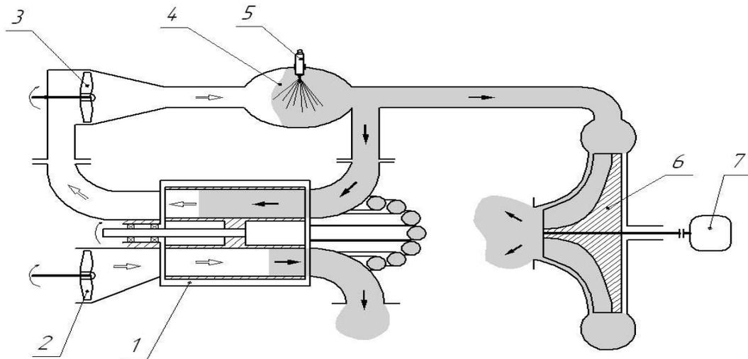
Fig.5. Diagram of gas- turbine unit with cascade pressure exchange
