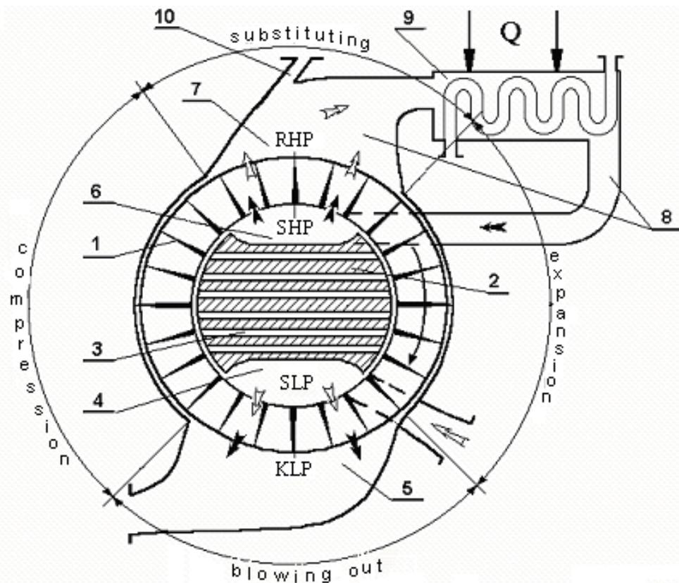
Fig.1. Fundamental diagram of cascade thermal compression compressor. 1 - rotor; 2- stator; 3- head interchange channels; 4, 5- supply window (SLP) and removal low pressure air [KLP]; 6, 7- supply window of high pressure air [SHP] and removal window of high pressure air [RHP]; 8- displayed path; 9- recover heat interchange; 10- branch pipe of compressed air removal to the consumer.
