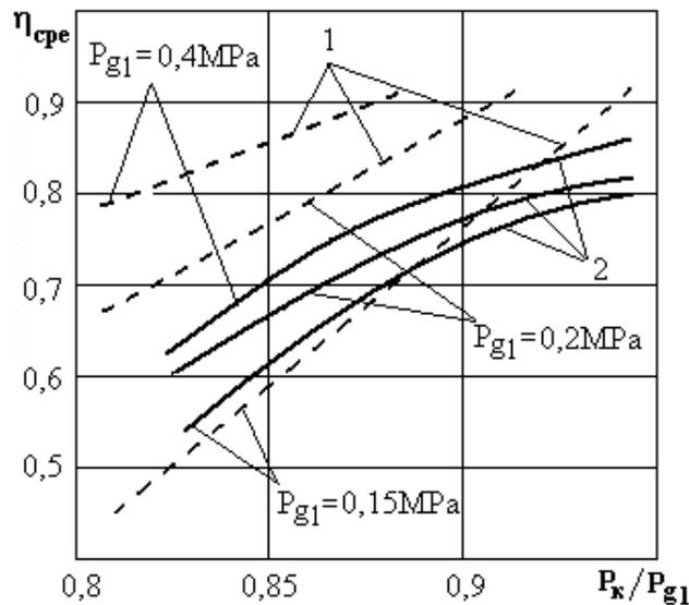
Fig.4. Efficiency dependency cascade pressure exchange on the ratio of pressure  $P_k/P_{g1}$
