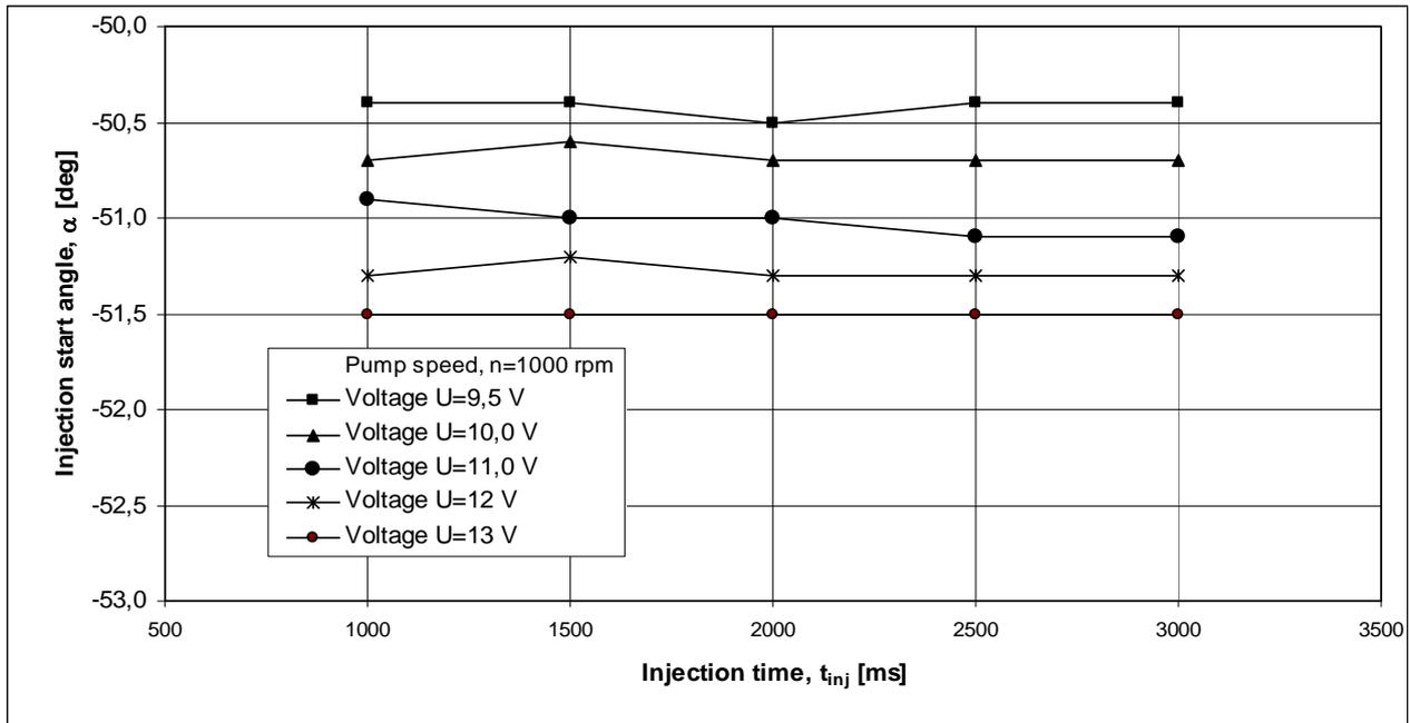
Fig. 4. Changes in the actual start of injection  $\alpha$  versus the injection time  $t_{inj}$  for different values of voltage  $U$  (the pressure in the rail  $p_{rail} = 75$  MPa,  $n = 1000$  rpm)
