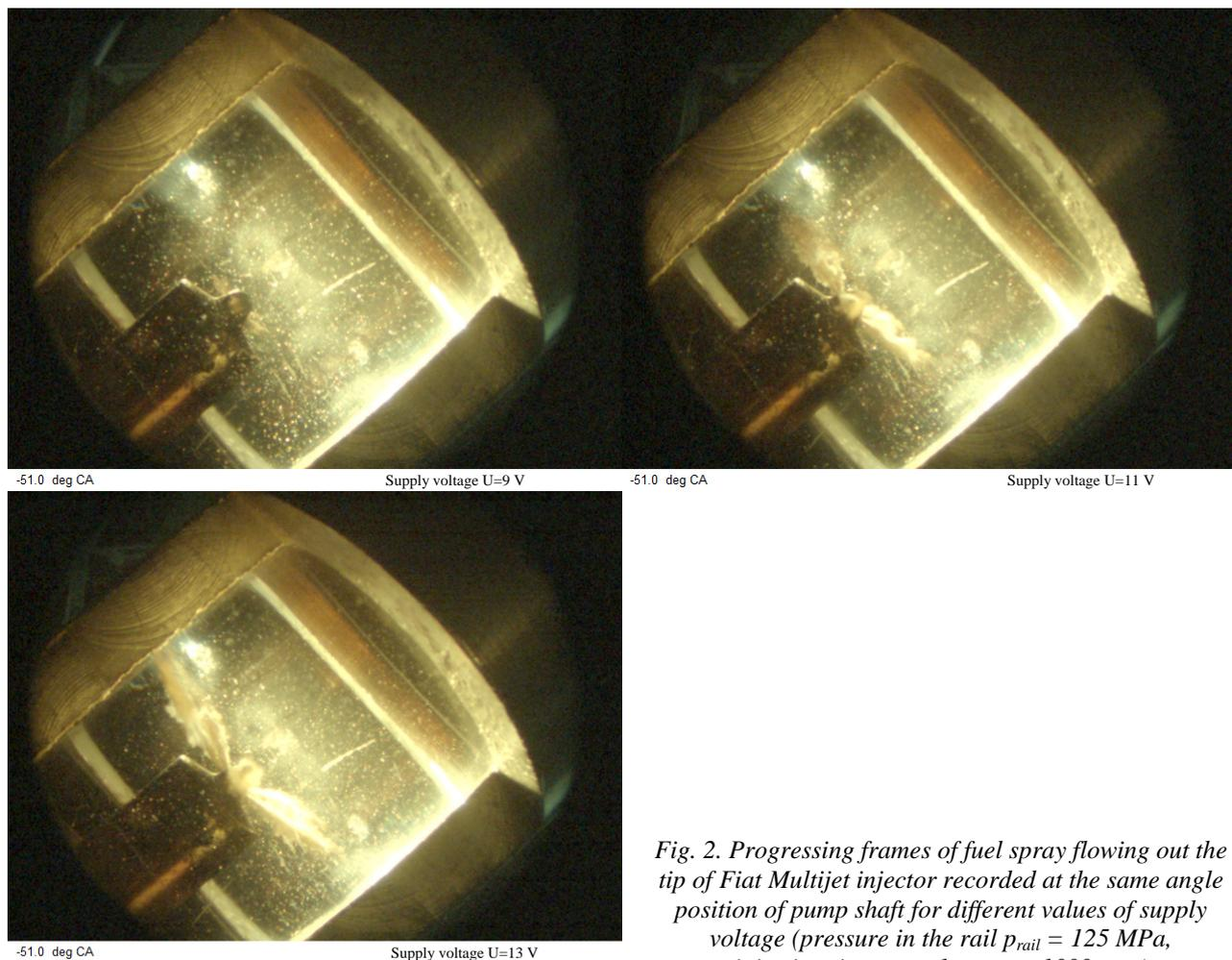
*Fig. 2. Progressing frames of fuel spray flowing out the tip of Fiat Multijet injector recorded at the same angle position of pump shaft for different values of supply voltage (pressure in the rail  $p_{rail} = 125 \text{ MPa}$ , injection time  $t_{inj} = 1 \text{ ms}$ ,  $n = 1000 \text{ rpm}$ )*
