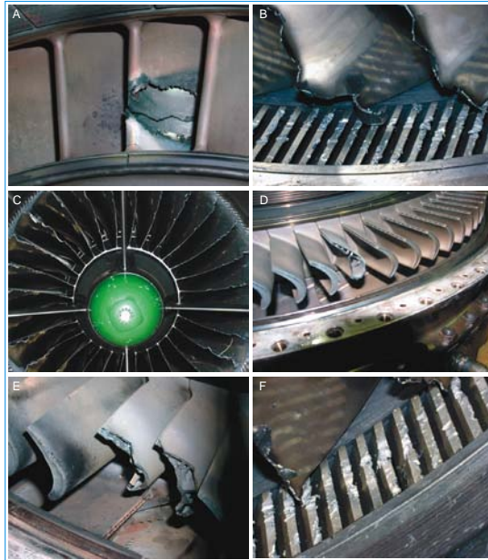
Fig. 3. Exemplary mechanical and heat-induced damages in the form of cracks and material defects in the turbine engine structure
