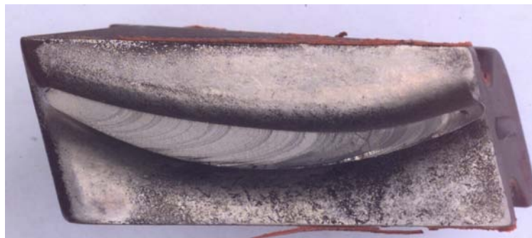
Fig. 7. Examples of fatigue failures to turbine engine's compressor blade
