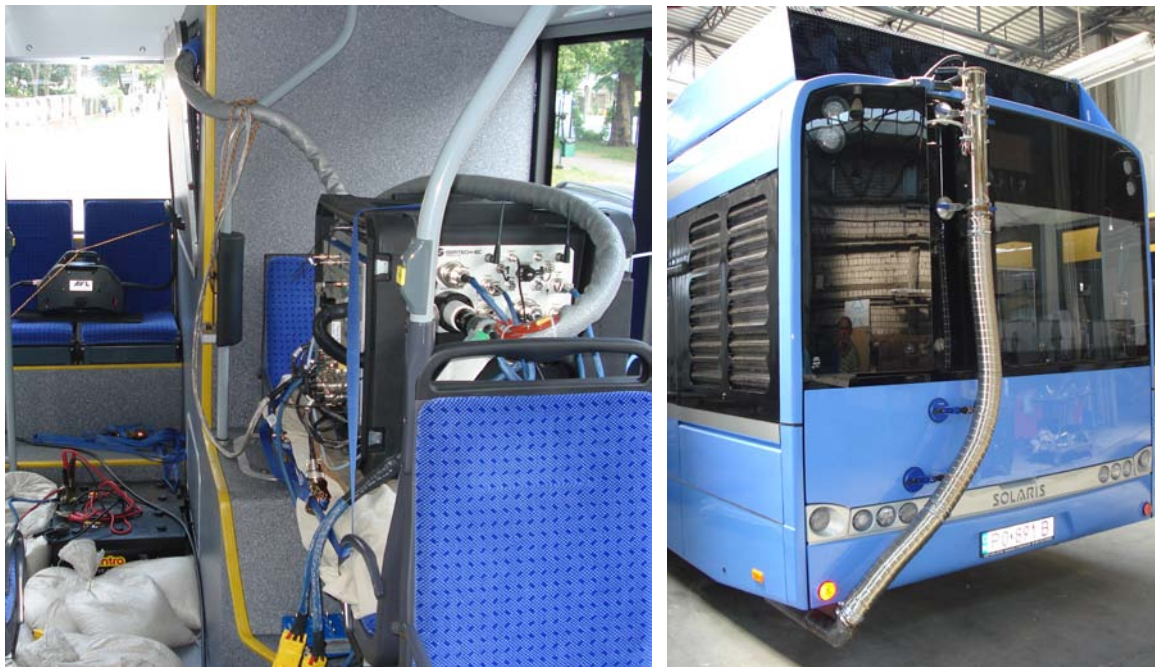
Fig. 2. View of the testing device (Semtech DS for exhaust emissions tests) fitted in the bus
