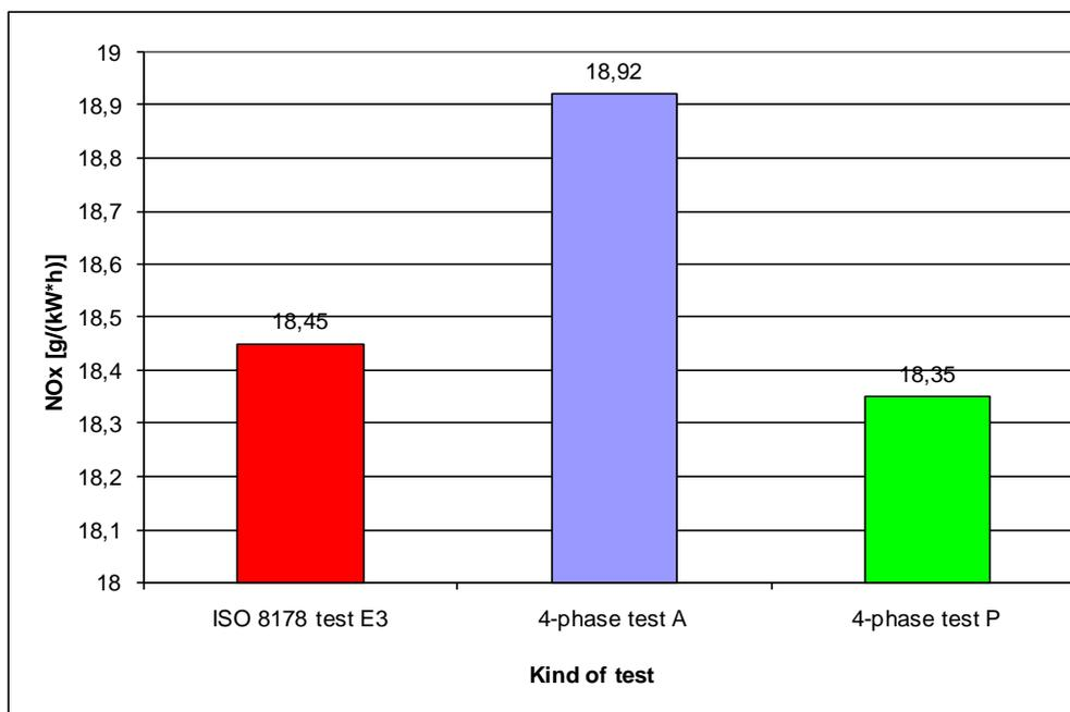
Fig.3. Comparison of  $NO_x$  emission values [g/(kW·h)] calculated by E3 test acc. to ISO 8170-4, 4-phase test A (required power  $P_0$  determined by Admiralty’s method) and 4-phase test P (required power  $P_0$  determined by Papiel’s method)
