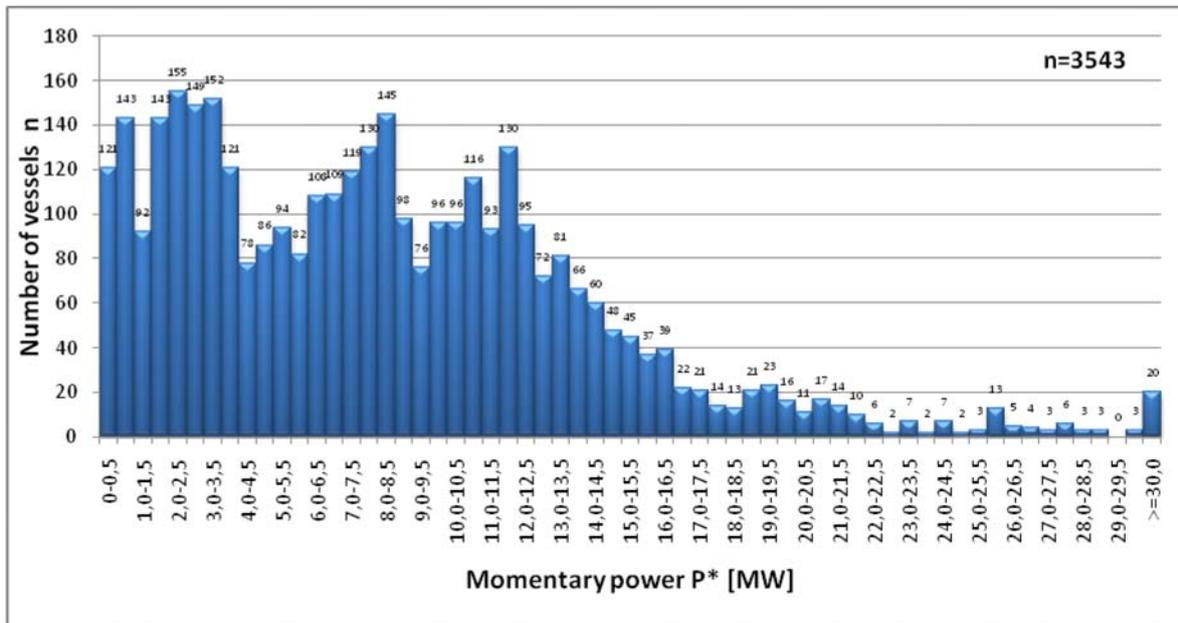
Fig. 1 Distribution of momentary power  $P^*$  [MW] calculated by Papiel's method for vessel group tested [9]
