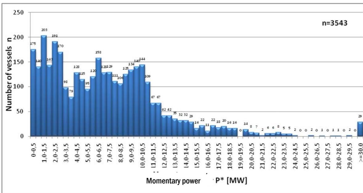
Fig. 2. Distribution of momentary power  $P^*$  [MW] calculated by Admiralty's method for vessel group tested [9]
