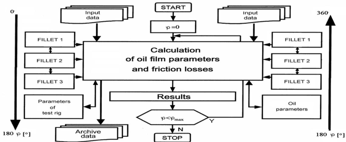
Fig. 6 Block schematic diagram of test stand mathematical model [5]
