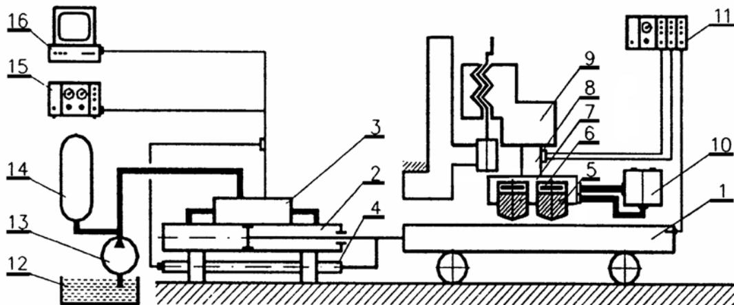
Fig. 3. Schematic of test stand: 1 – plate, 2 – actuator, 3 – control valve, 4 – position resistor, 5 – slat, 6 – flat spring, 7 – piston model, 8 – force transducer, 9 – support, 10 – slat pressure system, 11 – measuring&control system, 12 – hydraulic oil reservoir, 13 – oil pump, 14 – pressure accumulator, 15 – analogue control system, 16 – digital control system [5]
