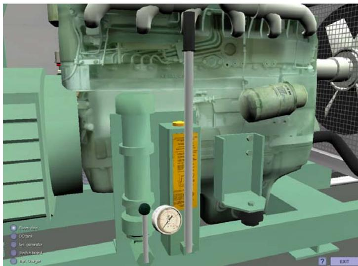
*Fig.5 Emergency hydraulic starter*
