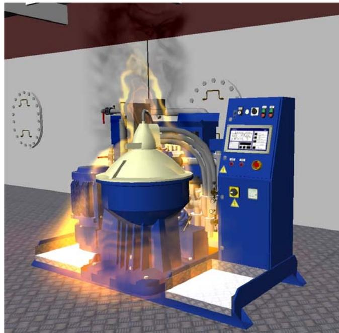
*Fig. 8 S-type fuel oil separator fire simulation*
