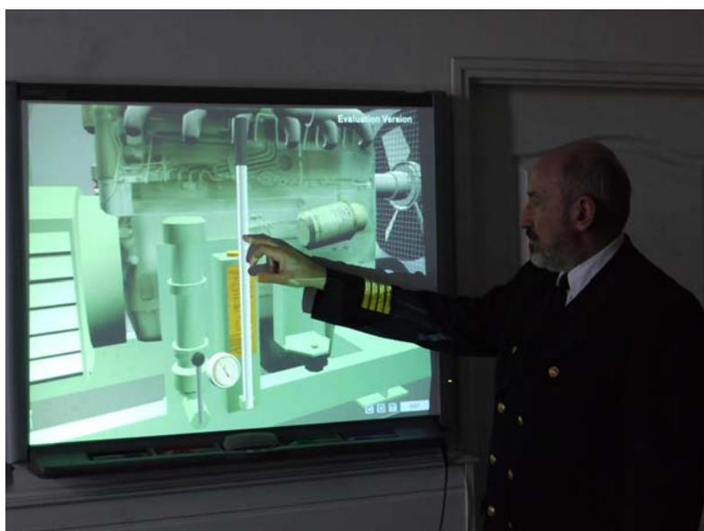
*Fig. 6 LER3D Engine Room Simulator – Application of touch screen for hydraulic starter emergency operation*
