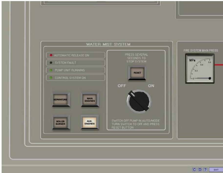
*Fig. 9 Water mist system – activation panel on engine control room*
