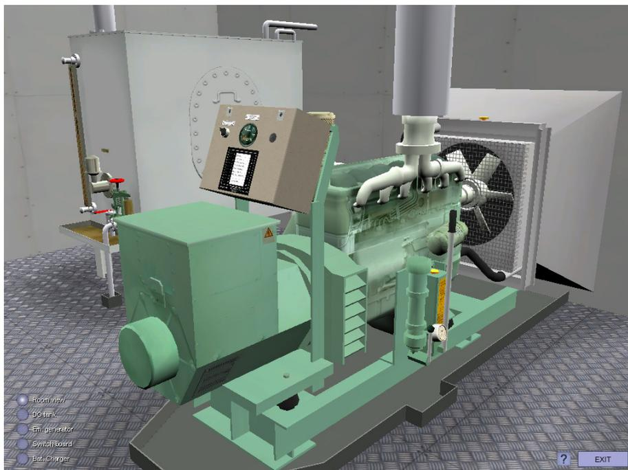
*Fig.4 Emergency Power Plant simulator - Diesel engine with control panel*
