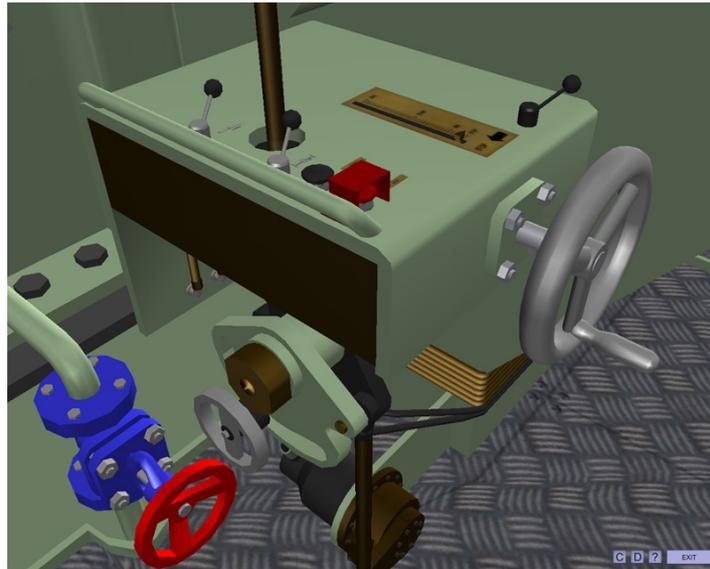
*Fig. 2 Low Speed Engine Room Simulator LER3D - Main engine emergency local control station*
