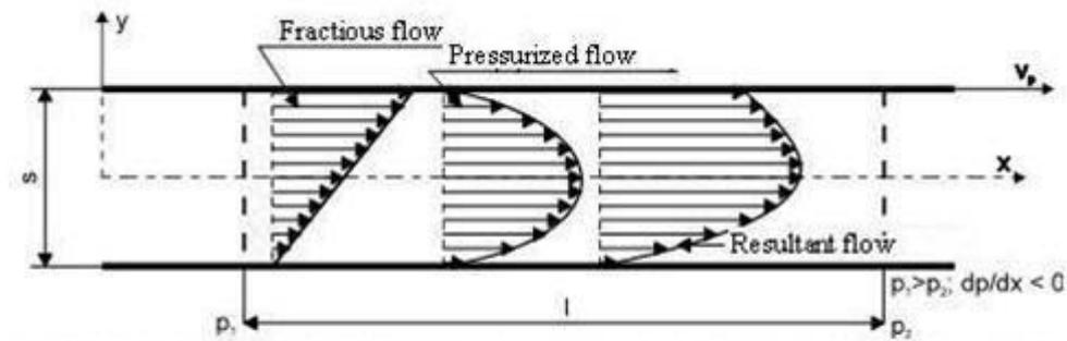
Fig. 2.4. Velocity distribution in the flat aperture at pressure difference and upper plate moving according to the direction of pressurized flow
