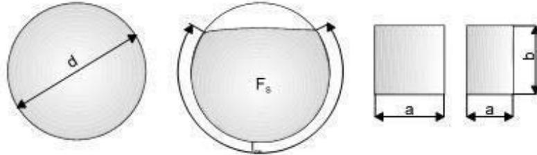
Fig. 2.6. The examples of hydraulic radiuses for the most common pipe sections
