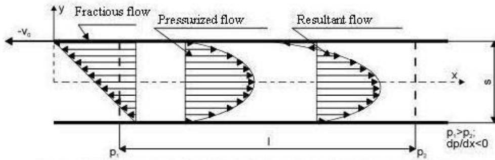
Fig.2,5. Velocity distribution in the total pressurized flow in the aperture at motion of upper plate opposite to the direction of pressurized flow
