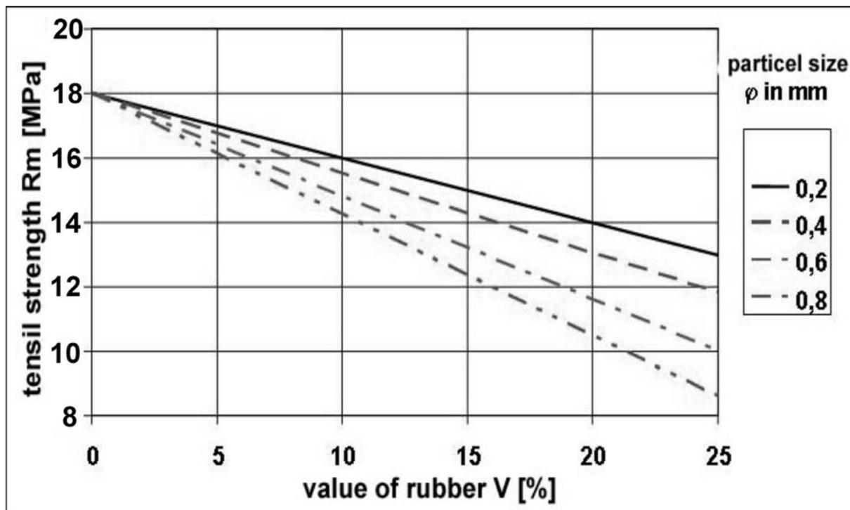
Fig. 3. Influence contents of rubber powder V[%] and sizes of grains(  $\varphi = 0.2; 0.4; 0.6$  and  $0.8$  mm) on endurance on extension  $R_m$  [MPa] – for injections
