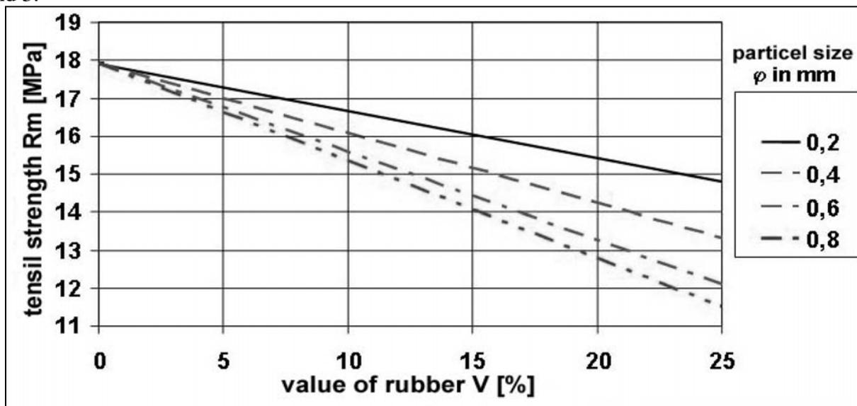
Fig. 2. Influence contents of rubber powder V[%] and sizes of grains(  $\varphi = 0.2; 0.4; 0.6$  and  $0.8$  mm) on endurance on extension  $R_m$  [MPa] – for pressing
