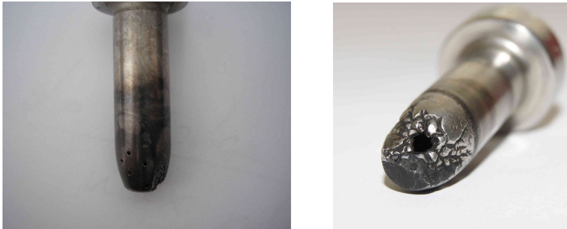
Fig. 6. Erosion-cavity formation damage together with local overheating (scorching) of the atomizer in a Sulzer RTA 58 engine
