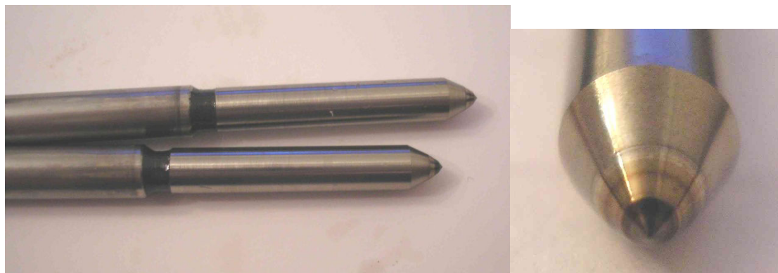
Figure 9 Scorched atomizer needle cones.
