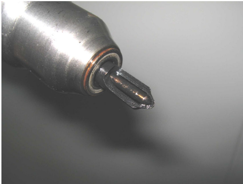
Fig. 4. A view of the damaged atomizer in a an injector pump of the Caterpillar engine
