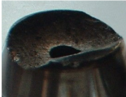
Fig. 1. Partial (fig. a) and total (fig. b) breakaway of the atomizer nipple
