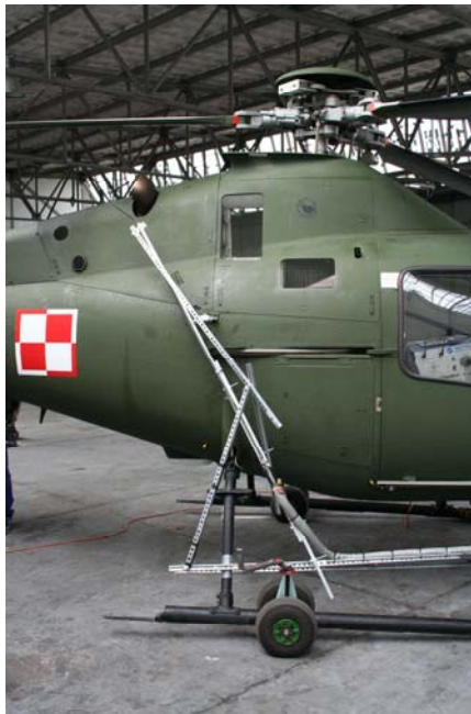
Fig. 3. Placement of the exhaust gases probe
