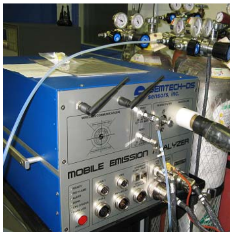
Fig. 4. View of the exhaust emission analyzer
