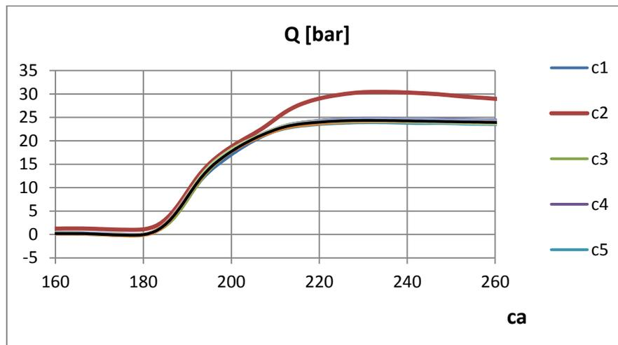
Fig. 3. Curves of net heat released in the cylinder  $Q$  for the measurement session C
