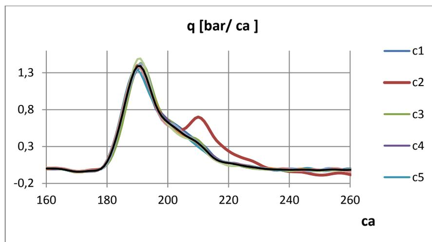
Fig. 4. The curve of heat release rate in the cylinders for the session C
