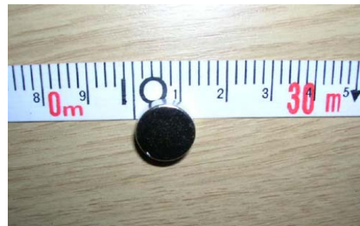
Fig. 5. The size of the magnet used for counterfeiting the indications of digital recording equipment
