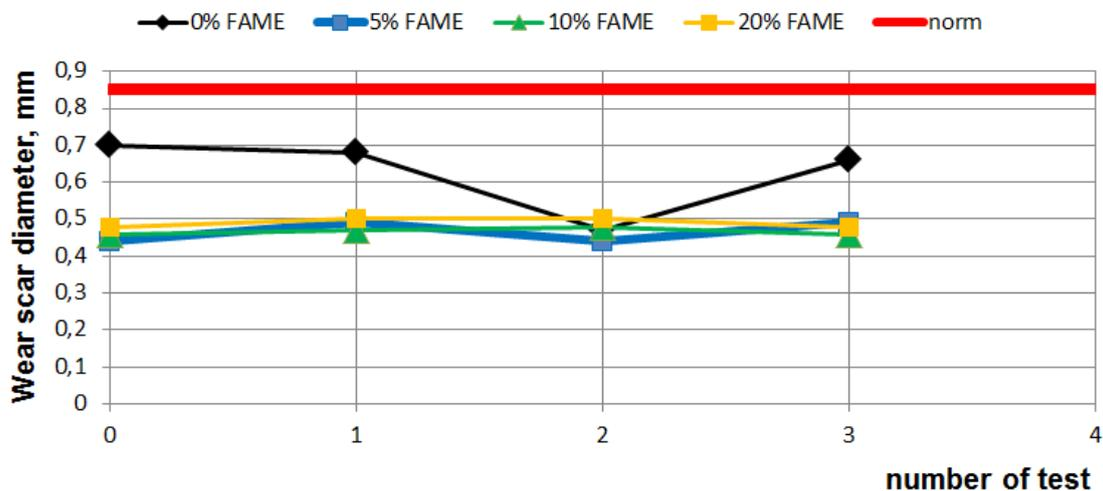
Fig. 2 Lubricity of aviation fuel and FAME blends (Type I) during storage
