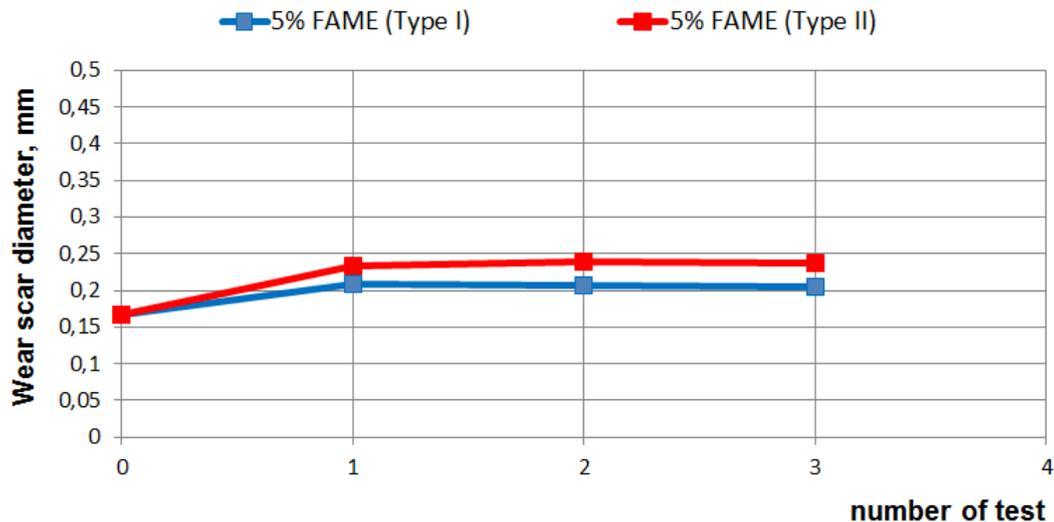
Fig. 8. Lubricity of selected blend of diesel fuel and FAME during storage depending on type of the blend
