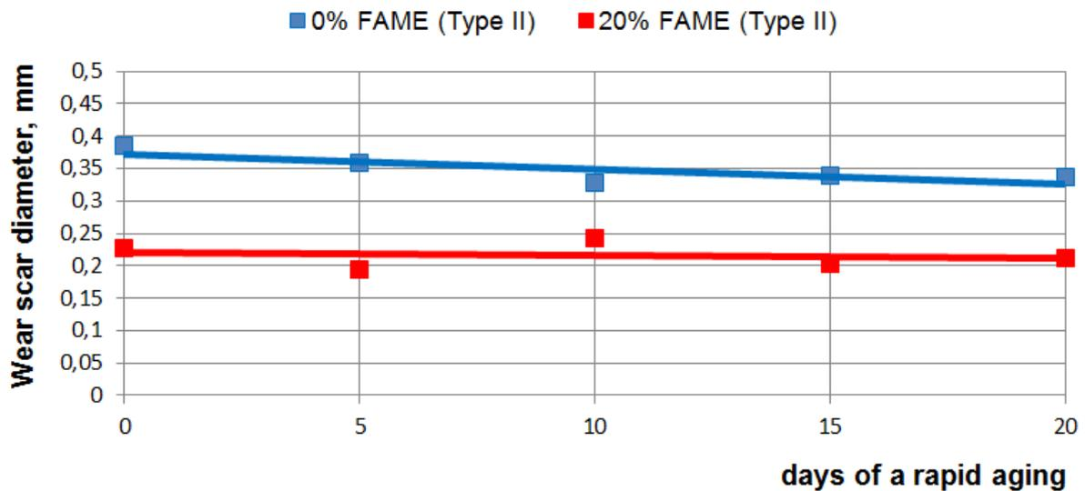
Fig. 1. Lubricity of selected diesel fuel and FAME mixtures during accelerated ageing
