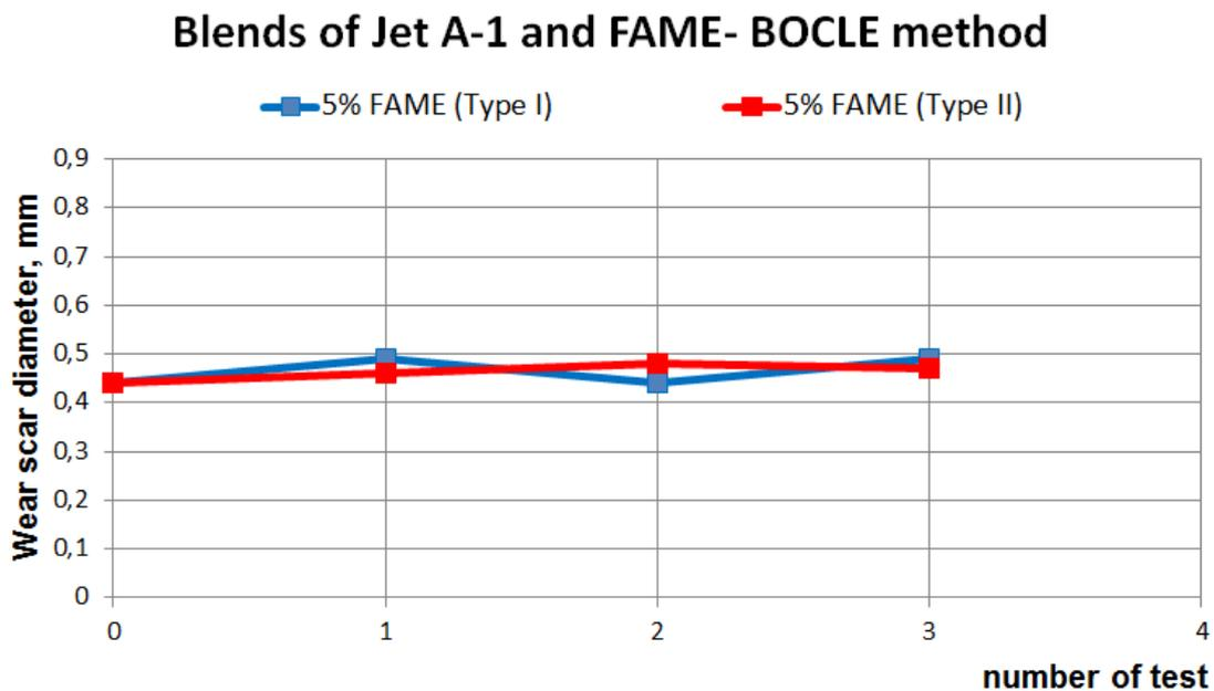
Fig. 7. Lubricity of selected blend of aviation fuel and FAME during storage depending on type of the blend
