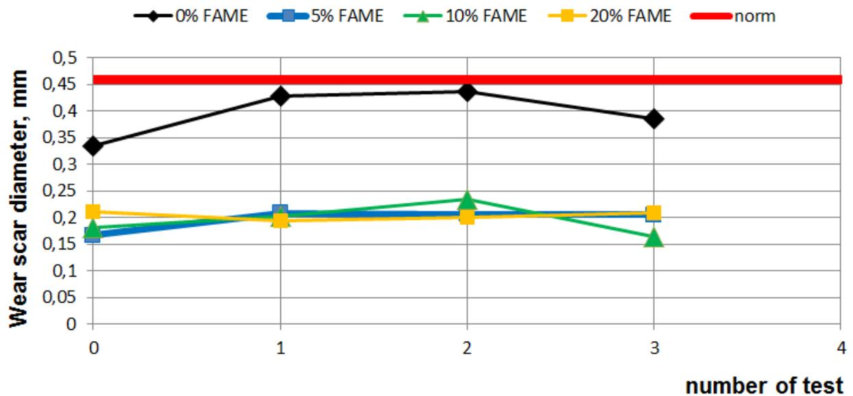
Fig.4. Lubricity of diesel fuel and FAME blends (Type I) during storage
