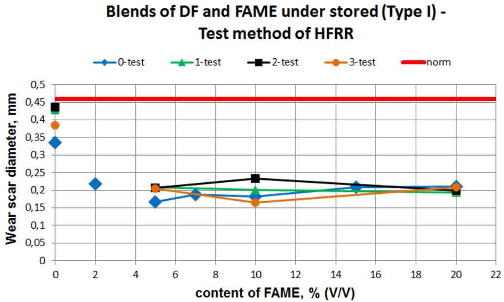
Fig. 6 Lubricity of mineral fuels and FAME blends (Type I) during storage
