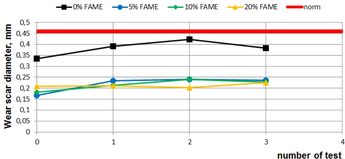
Fig. 5. Lubricity of diesel fuel and FAME blends (Type II) during storage
