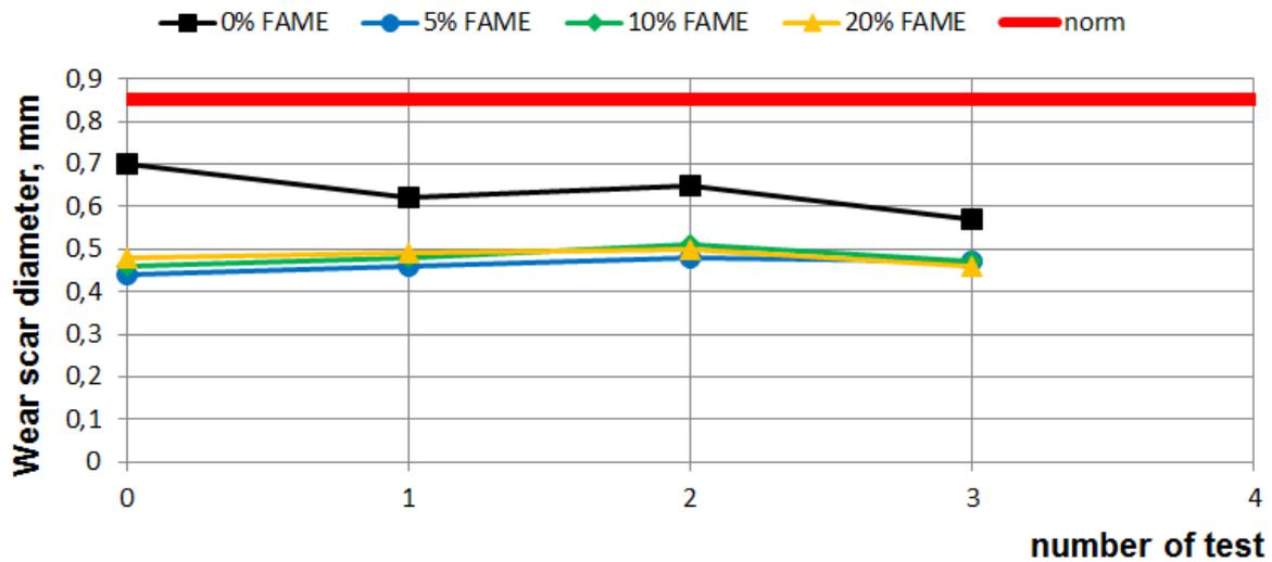
Fig. 3 Lubricity of aviation fuel and FAME blends (Type II) during storage
