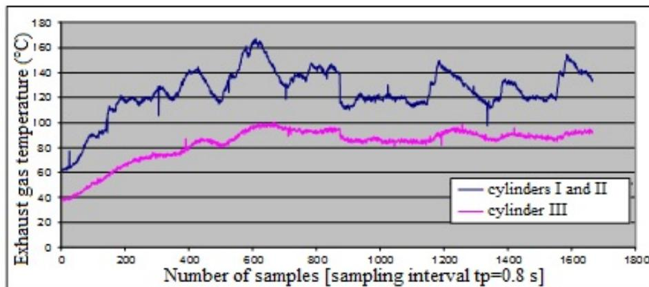
Fig. 8. Changes in exhaust gas temperature in each cylinder over time
