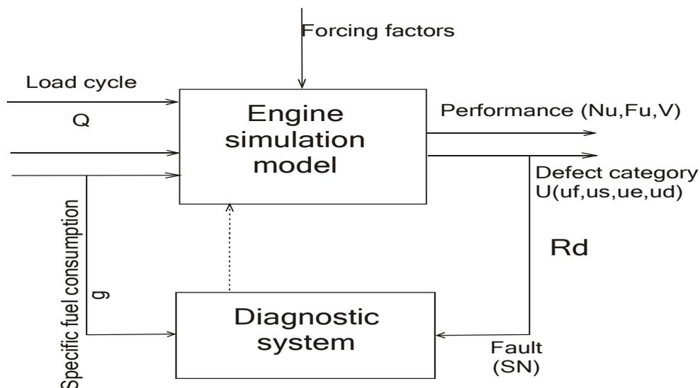
Fig. 2. Diagnostic diagram of a wheeled tractor based on the proposed mechatronic system for monitoring the condition of wheeled tractor (MSMC), where:  $g$  – specific fuel consumption,  $S_N$  – fault,  $U$  – defect category [4]
