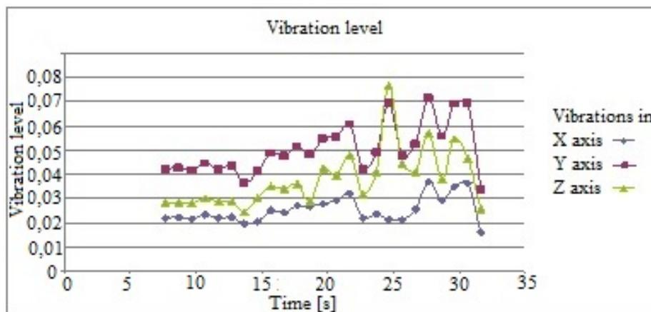
Fig. 10. Changes in engine vibration levels over time
