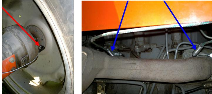
Fig. 6. Rear wheel rotational speed sensor (left) and exhaust gas temperature sensor (right) [Photograph by Jaroslaw Gonera]
