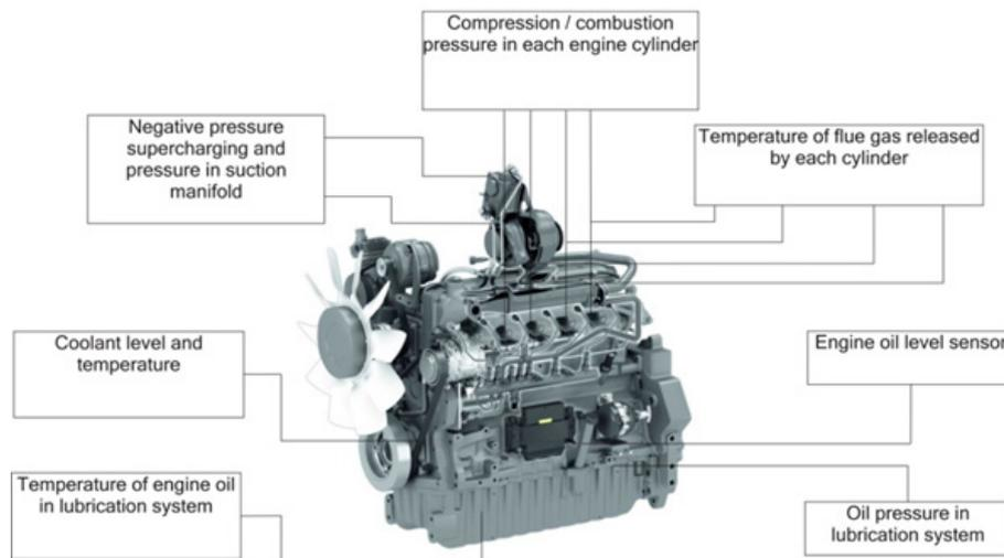
Fig. 4. Distribution of sensors for monitoring engine operation in a wheeled tractor [9]
