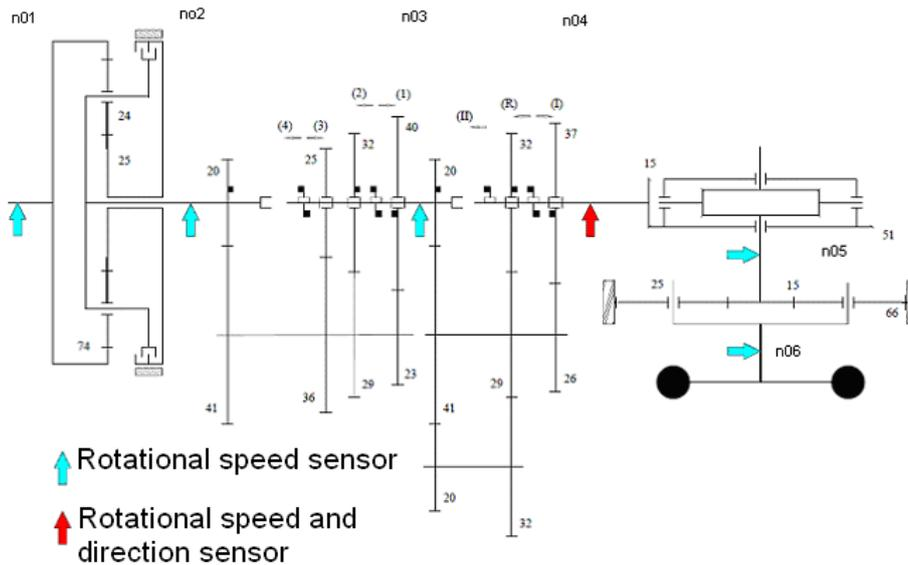
Fig. 3. Distribution of diagnostic sensors in a kinematic diagram of a tractor's power transmission system
