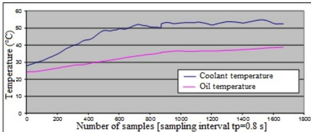
Fig. 9. Changes in the temperature of the coolant and engine oil over time
