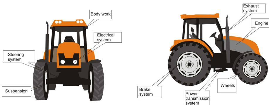
Fig. 1. Diagram of the main components and systems in a wheeled tractor
