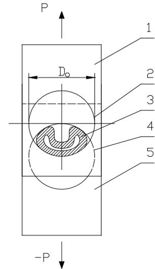
Fig.2: Intensive deformations (relations) model of pipe's as recycling element;  $v_R = 0.01 \text{ m} \cdot \text{s}^{-1}$  (except for rigid PVC-waste), 1 - motionless slat, 2 - draft of the hole in motionless slat; 3 - investigated sample; 4 - draft of the hole in moveable slat; 5 - moveable slat.
