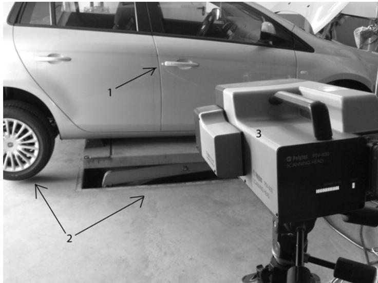
Fig. 3. Test rig: 1– place from which laser beam is reflected, 2 – method of isolating from base (jacking up), 3 – scanning probe
