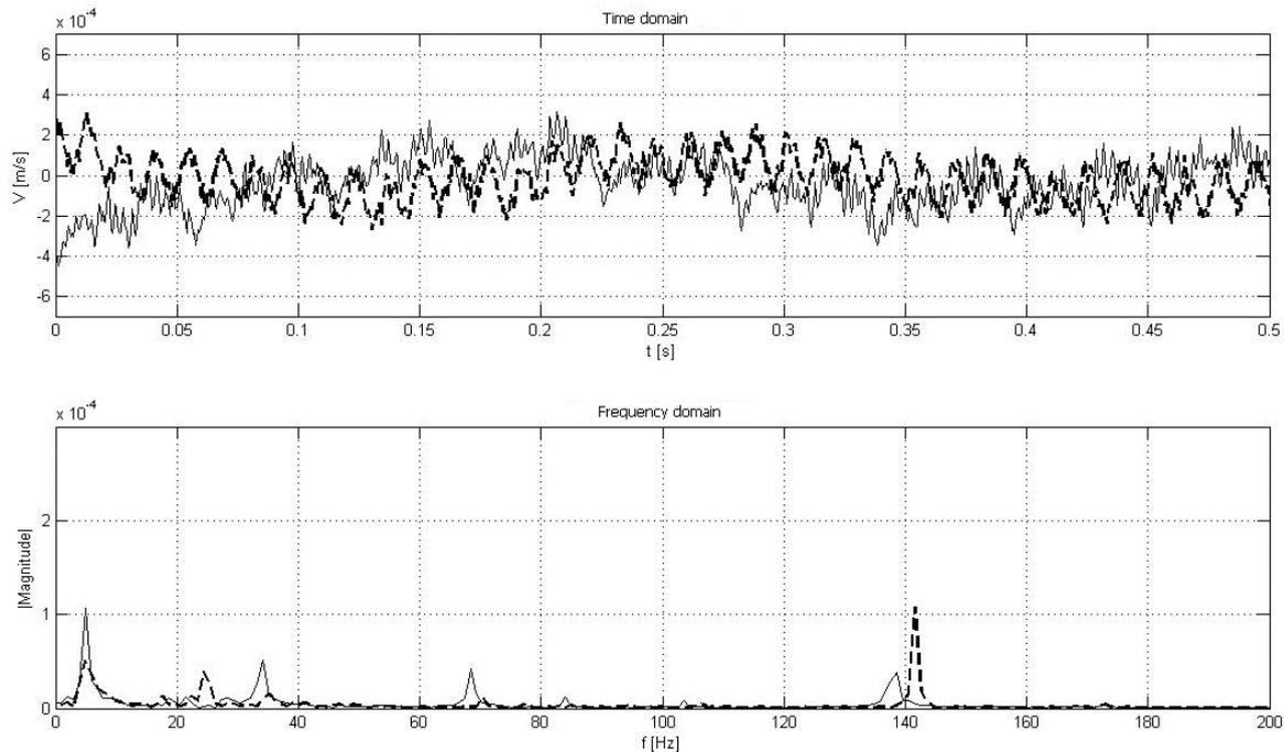
Fig. 5. Waveform and frequency spectrum of vibration velocities measured behind passenger handle for jacked up idle running ( $2000 \text{ rpm}$ ) car; solid line is for car having engine equipped with supercharger
