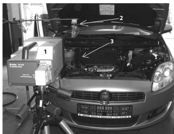
Fig. 2. Test rig: 1- laser probe, 2- mirror, 3- place of laser beam reflection
