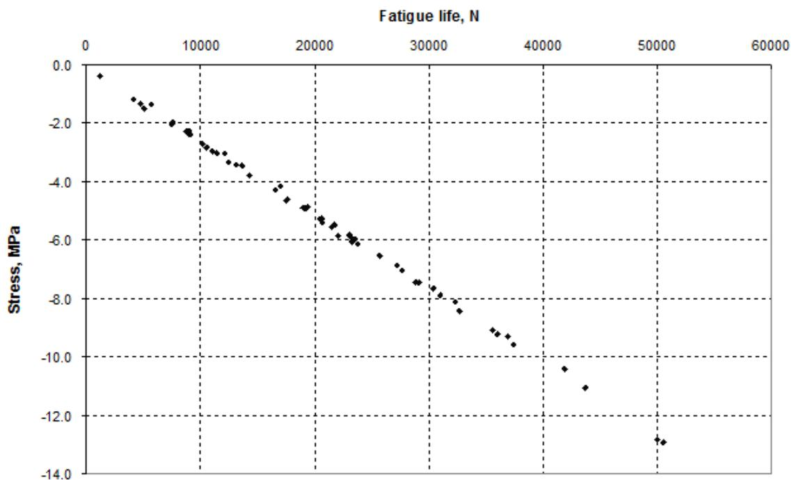
Fig. 2. Fatigue life versus maximal compression stress
