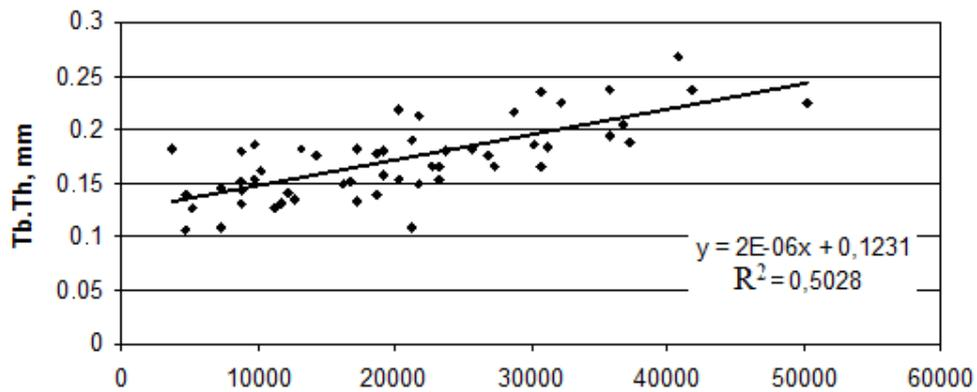
Fig. 4. Relationship between fatigue life  $N$  and trabecular thickness  $Tb.Th$
