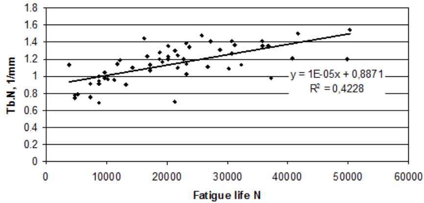
Fig. 5. Relationship between fatigue life N and trabecular number Tb.N
