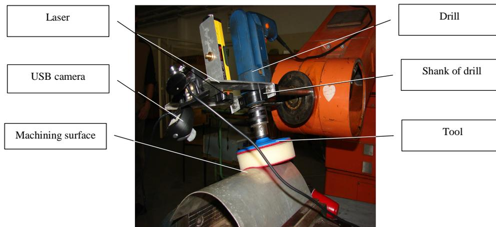
Fig. 8. View system in surface finish machining
