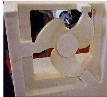
Fig. 3. Example of milling mold surface [10]
