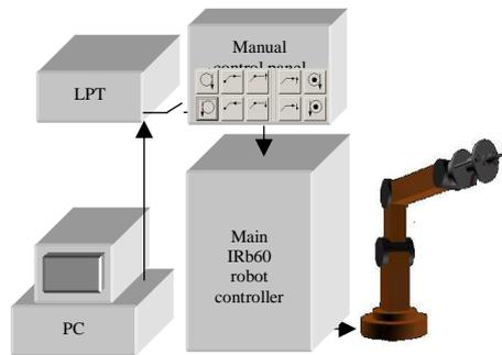
Fig. 5. IRb60 robot control system using PC [7]
