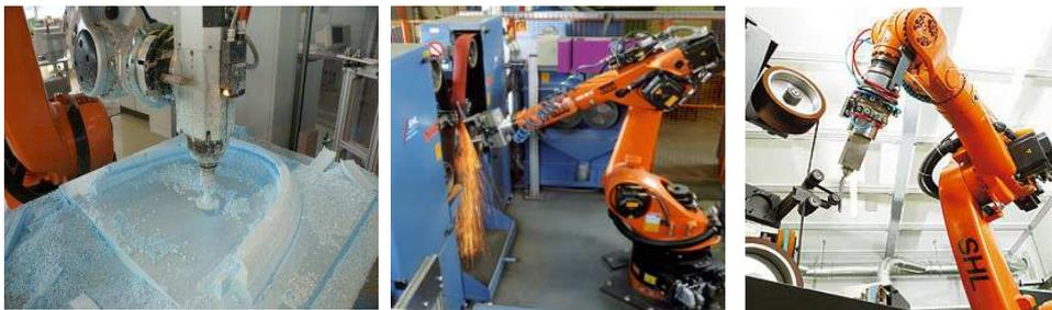
Fig. 1. Robot machining: a) milling [9], b) grinding [9], polishing [11]
