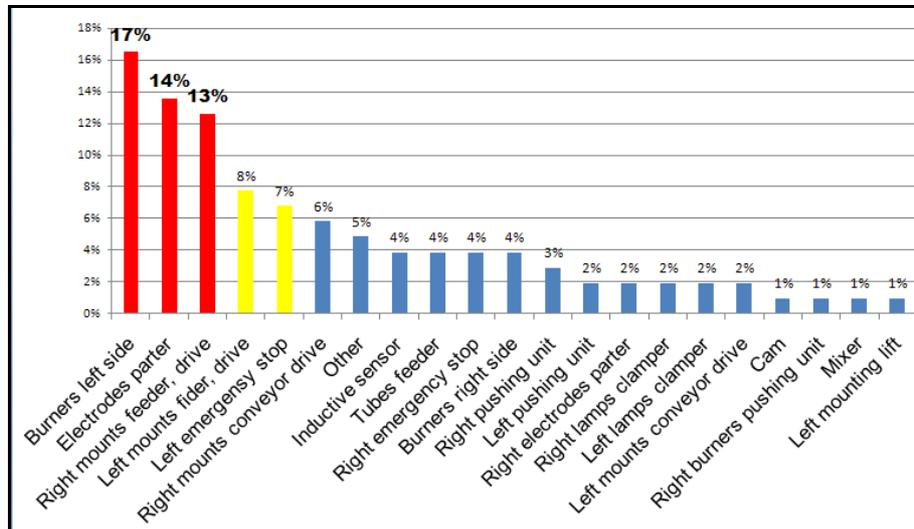
Fig.7. Breakdowns probability of sealing machines units
