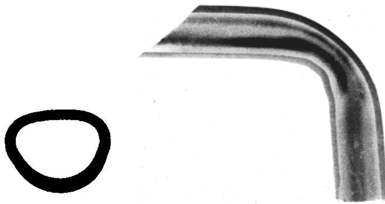
Fig. 10. Section of the pipe - experimental test
