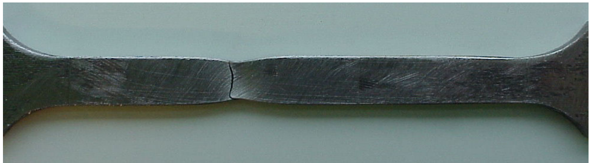
Fig. 5. Shape of damage of specimen with weld
