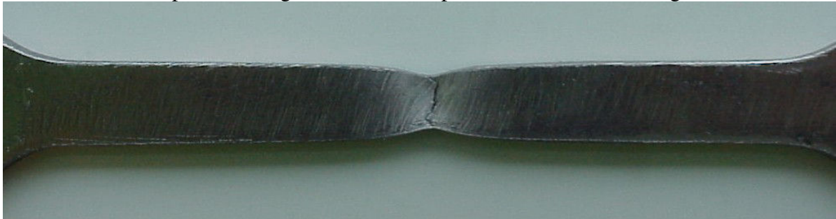
Fig. 4. Shape of damage of specimen without welds
