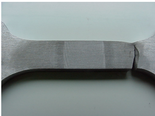
Fig 6. Shape of cracks in specimens with welds in the measuring part of the specimen
