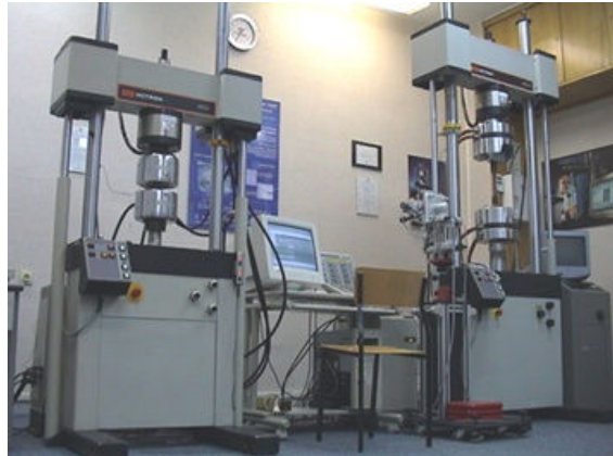
Fig. 2. INSTRON servo-hydraulic material-testing machines, laboratory of University of Technology and Life Science
