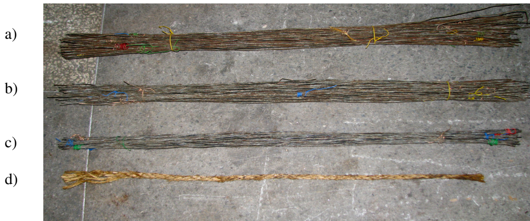
Fig.4. Prepared for tests segments of wires of the rope layers: a) external, b) central, c) internal and d) core
