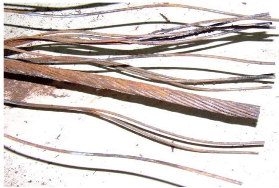
Fig. 2. Some fragment of the rope before the tests with visible corrosion
