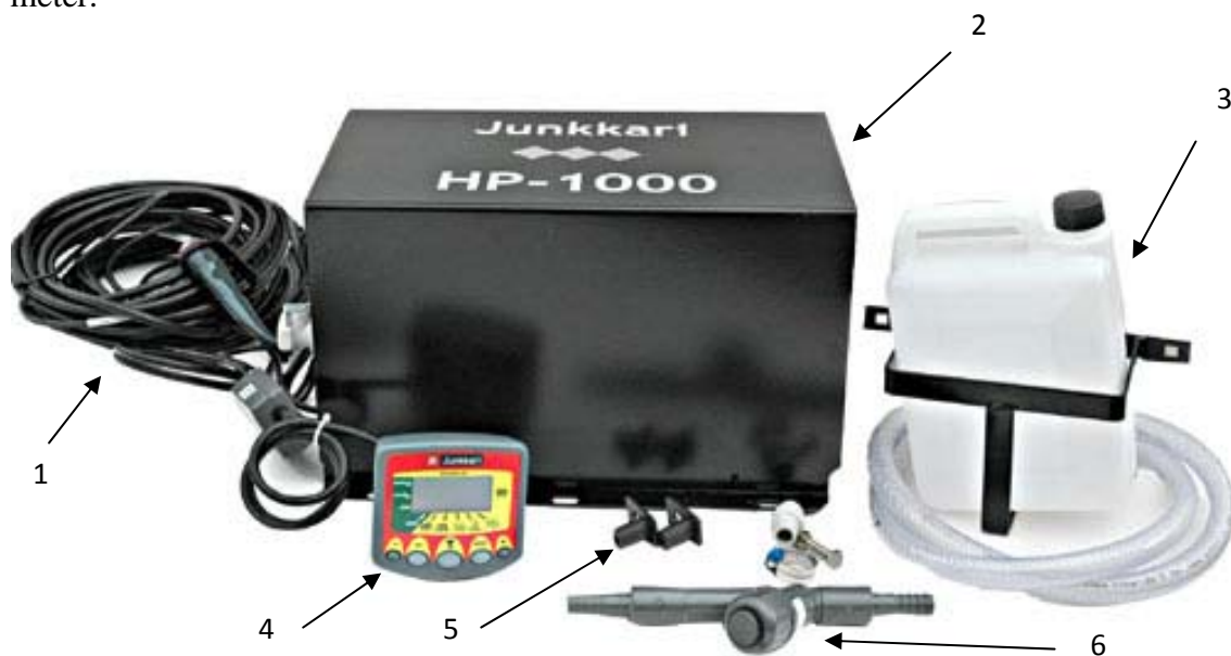
Fig. 1. Picture of HP 100 dosing installation of Junkkari company: 1 – cords; 2 – membrane pump with a flow-meter; 3 – container with a preservative with an elastic conduit; 4 – controller; 5 – nozzle; 6 – leak protection valve
