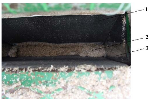
Fig. 2. Folding chamber shape in the initial phase of work (top view): 1 - wrapper, 2 - coiled material, 3 - lateral ventricle wall collapse
