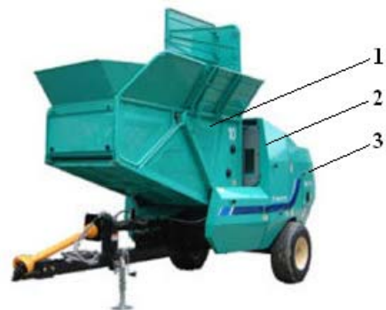
Fig. 5. Japanese business newspaper Takakita Co. Ltd model MR 810: 1-receiving basket, 2- the front part of the chamber collapse, 3-back, moving part of the chamber collapse
