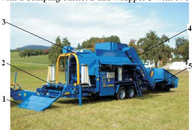
Fig. 4. Baler Göweil LT-Master: 1-unloading ramp, 2-wrapper, 3-chamber collapse, 4-inclined conveyor, 5-receiving basket
