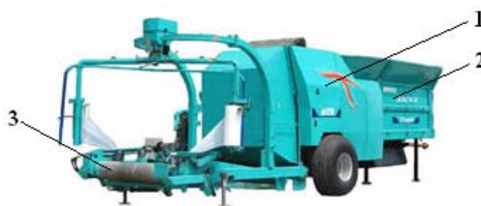
Fig. 6. Japanese business newspaper Takakita Co. Ltd model MW 1220: 1-chamber collapse, 2-hopper, 3-wrapper, with two rotating arms
